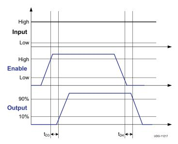
Figure 1. Enable Function
