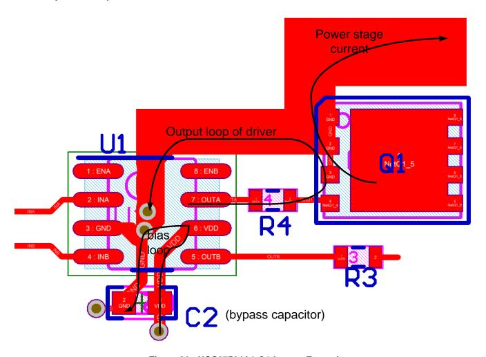
Figure 30. UCC27524A1-Q1 Layout Example
