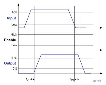
Figure 2. Input-Output Operation
