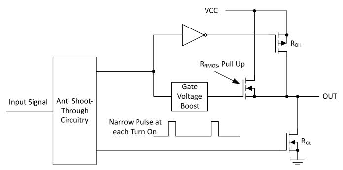
Figure 20. UCC27524A1-Q1 Gate Driver Output Structure
