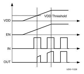
Figure 27. Power-Up Non-Inverting Driver
