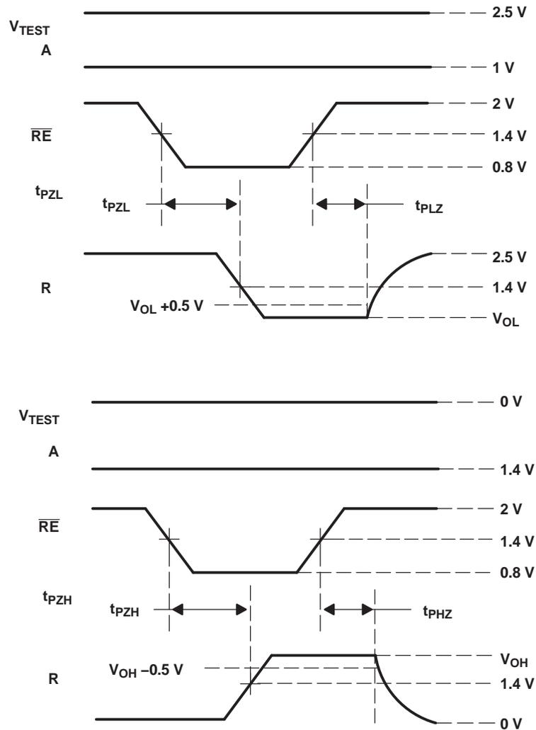
Figure 7. Enable/Disable Time Test Circuit and Waveforms
