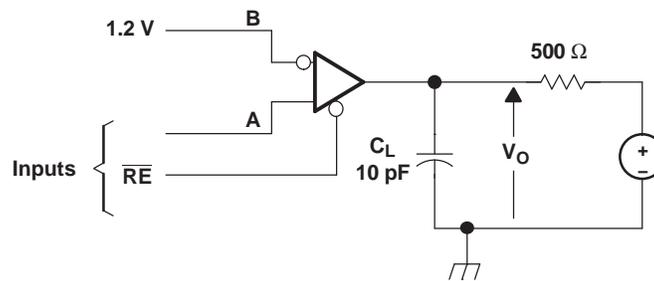
NOTE A: All input pulses are supplied by a generator having the following characteristics:  $t_r$  or  $t_f \leq 1$  ns, pulse repetition rate (PRR) = 0.5 Mpps, pulse width =  $500 \pm 10$  ns.  $C_L$  includes instrumentation and fixture capacitance within 0,06 mm of the D.U.T.
