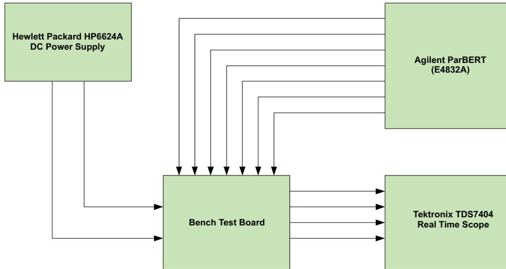
Figure 16. Equipment Setup
