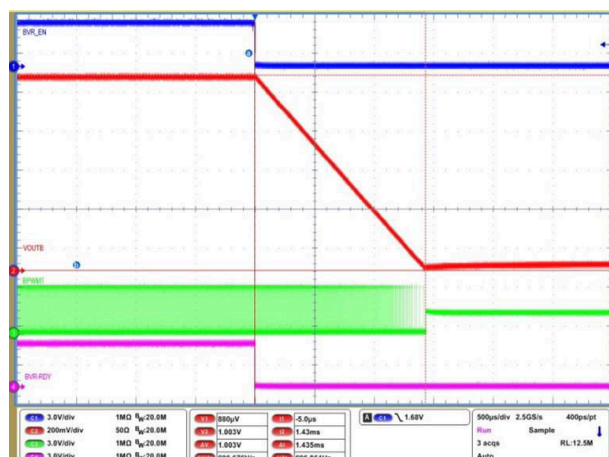
Figure 8-20. Soft-stop channel B (0 ms TOFF_DELAY)
