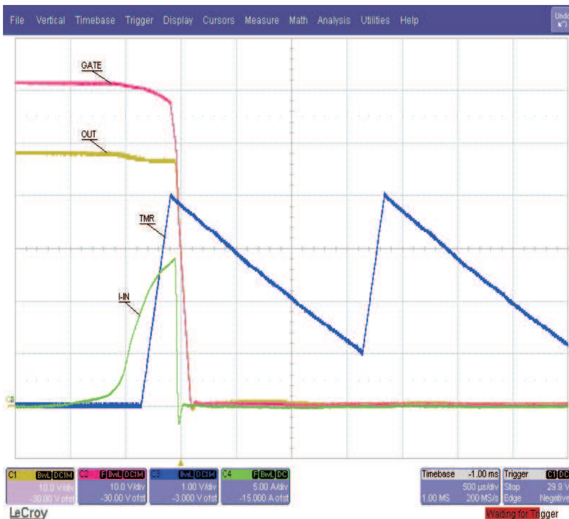
Figure 16. TPS2480/81 Restart Cycle Timing
