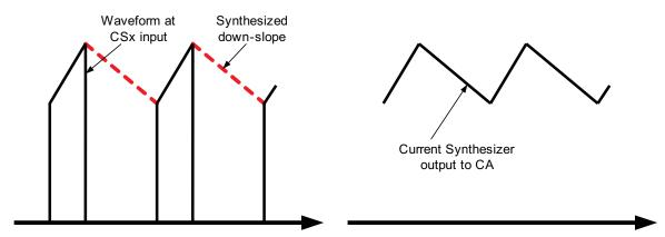
Figure 19. Downslope of the Inductor Current
