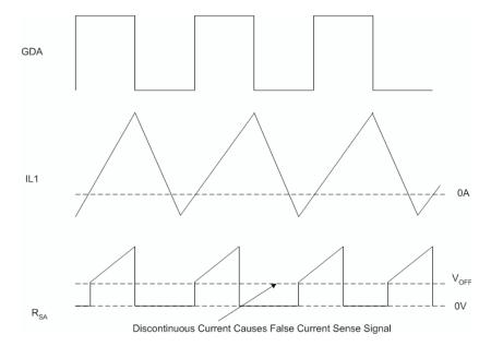
Figure 28. False Current Sense Signal
