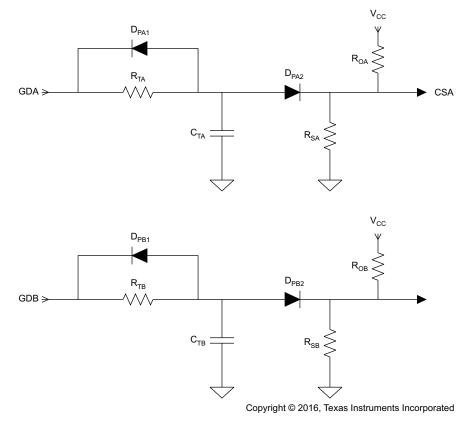
Figure 27. PWM Ramp and Offset Circuit
