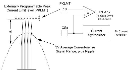
Figure 20. Externally Programmable Peak Current Limit
