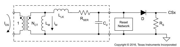
Figure 25. Current Sense Transformer Equivalent Circuit
