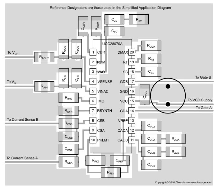
Figure 33. Layout Diagram
