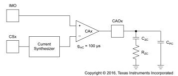
Figure 22. Current Error Amplifier With Type II Compensation
