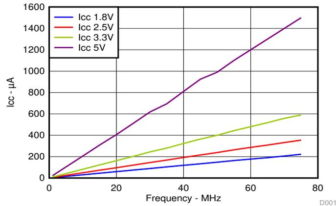
**Figure 5. I<sub>CC</sub> vs Frequency**
