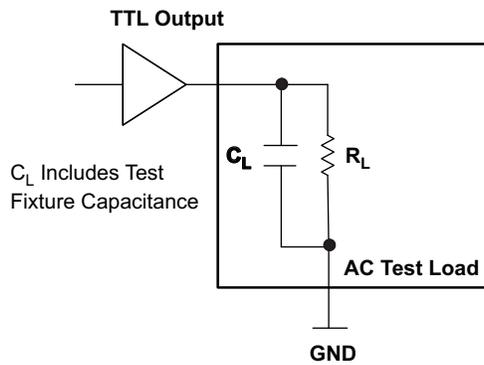
Figure 1. TTL Output AC Test Loading Condition
