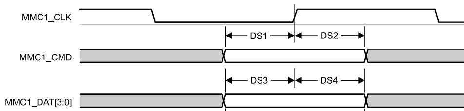
Figure 7-96. MMC1/2 – Default Speed – Receive Mode
