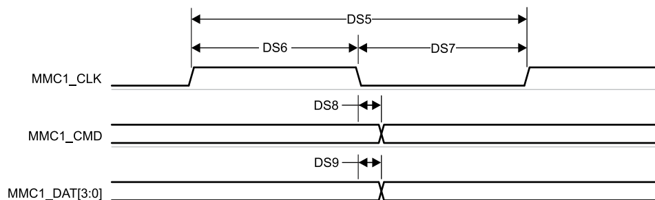
Figure 7-97. MMC1/2 – Default Speed – Transmit Mode
