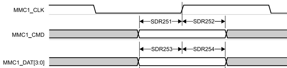
Figure 7-102. MMC1/2 – UHS-I SDR25 – Receive Mode
