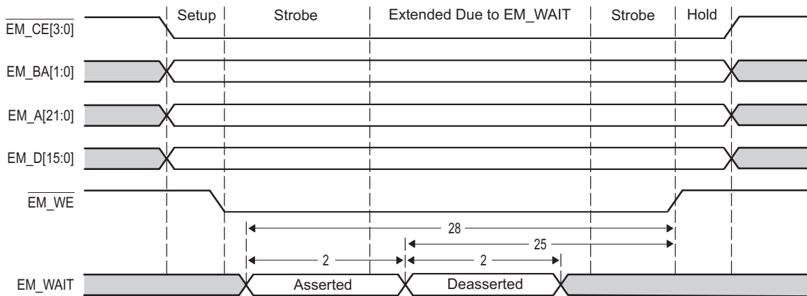
图 11-56. EMIF16 EM_WAIT Write Timing Diagram
