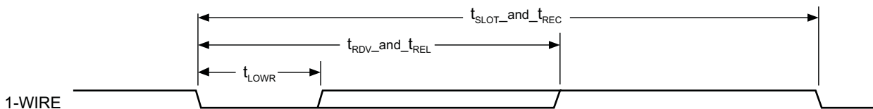
图 7-30. 1-Wire—Read Bit (Data)
