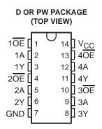
The SN74AHCT125 is a quadruple bus buffer gate featuring independent line drivers with 3-state outputs. Each output is disabled when the associated output-enable (OE) input is high. When OE is low, the respective gate passes the data from the A input to its Y output.
