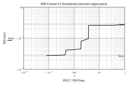
Figure 1. VDD Current Consumption
