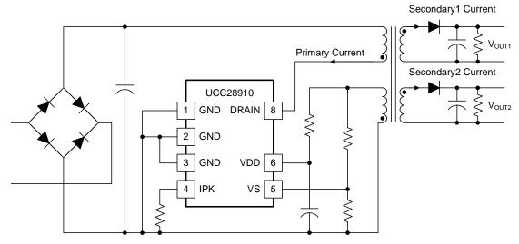
Figure 49. Multi-Output Flyback Converter
