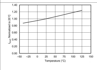
Figure 18.  $I_{WAIT}$  vs Temperature
