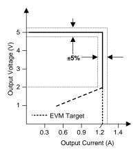
Figure 33. Target Output V-I Characteristic
