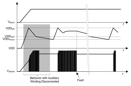
Figure 30. Start Up and Auto Re-Start Operation
