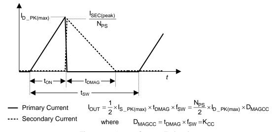
Figure 23. Output Current Estimation
