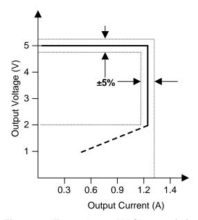
Figure 24. Target Output V-I Characteristic
