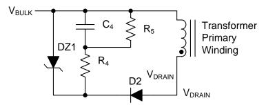
Figure 40. DRAIN Clamp Circuit Options
