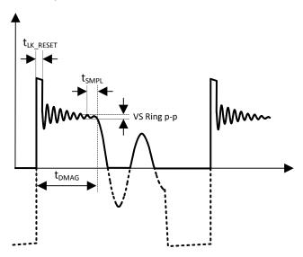
Figure 22. VS Voltage
