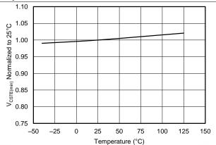
Figure 8. UCC28910  $V_{CSTE(min)}$  vs Temperature
