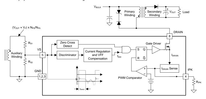
Figure 25. Output Current Control Loop Block Diagram
