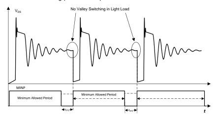
Figure 29. Valley Switching Disable at Light Load
