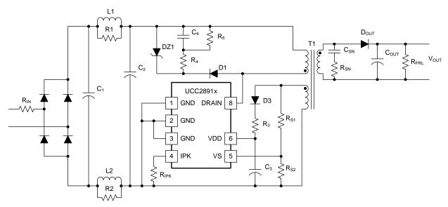
Figure 35. Standard Flyback Converter Based on UCC2891x
