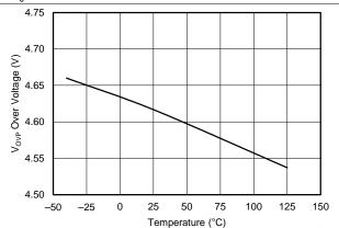
Figure 14. V<sub>VSR</sub> vs Temperature
