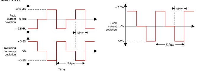
Figure 31. EMI Dithering During CV Mode Operation
