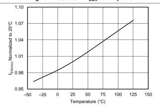
Figure 12.  $f_{SW(max)}$  vs Temperature
