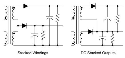
Figure 51. Stacked Windings and DC Stacked Outputs
