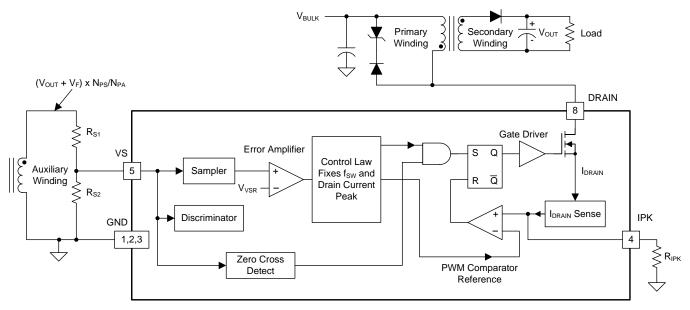
Figure 20. Voltage Loop Block Diagram
