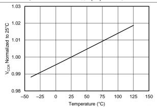
Figure 10. UCC28910 V<sub>CCR</sub> vs Temperature
