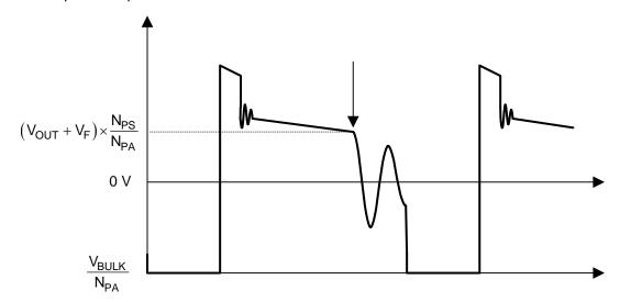
Figure 21. Auxiliary Winding Voltage
