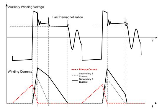
Figure 50. Winding Current Waveform in Multi-Output Flyback Converter
