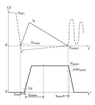
Figure 1. Typical Waveforms of APR340 in DCM
