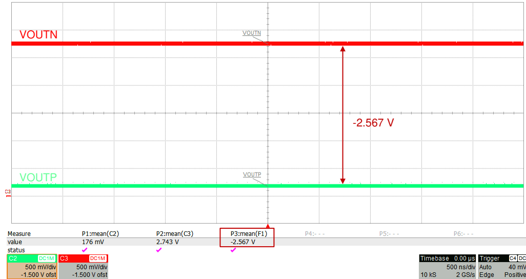
图 7-5. Typical Failsafe Output of the AMC3301
