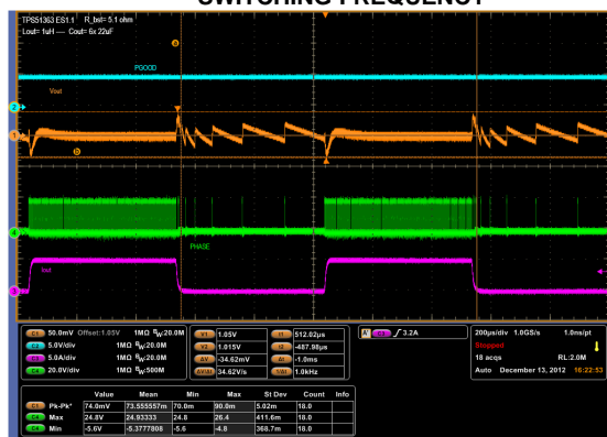
Figure 21. f = 400\text{kHz} , V_{IN} = 20\text{V} , I_{OUT} = 0-5\text{A}
