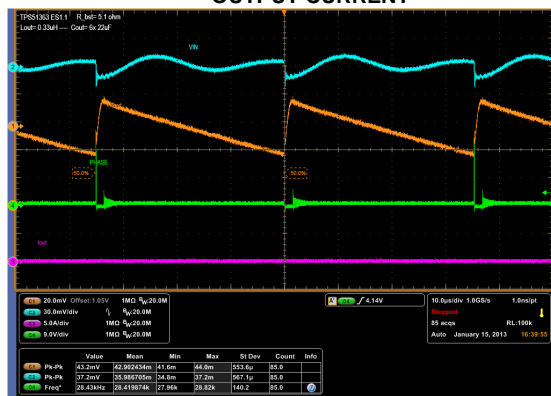
Figure 19. f = 800\text{kHz} , V_{IN} = 20\text{V} , I_{OUT} = 0.1\text{A}
