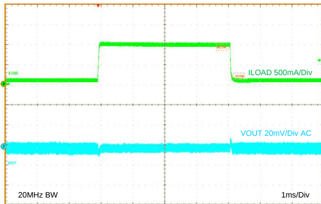
Figure 60. Load Transient V_{OUT} = 3.3\text{ V}
