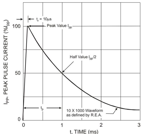
Fig. 2 Pulse Waveform
