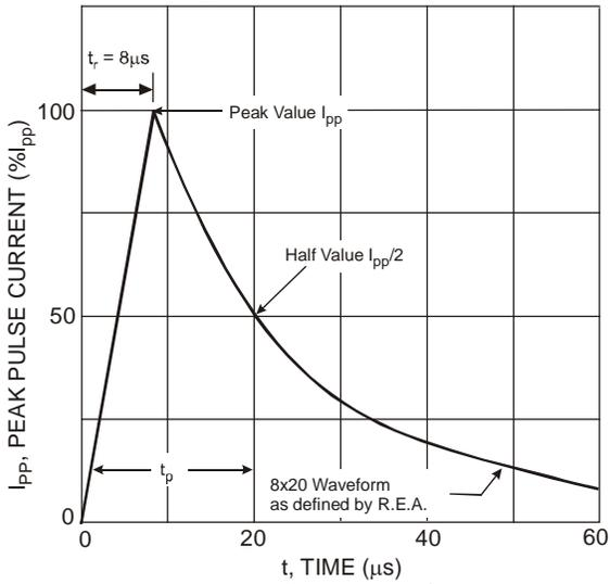
Figure 3 Pulse Waveform
