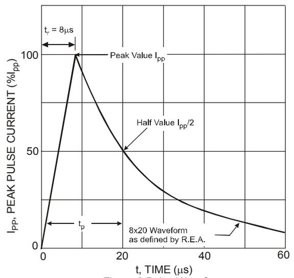
Figure 2 Pulse Waveform
