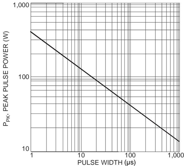
Fig. 5 Pulse Rating Curve vs. Pulse Width
