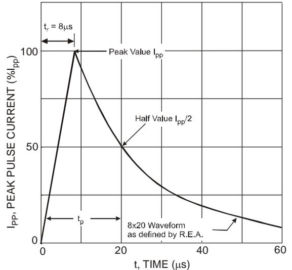
Fig. 2 Pulse Waveform
