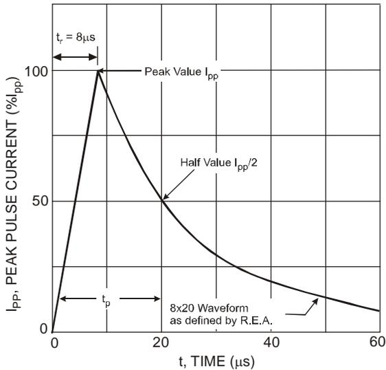
Figure 3 Typical 8 x 20µs Pulse Waveform
