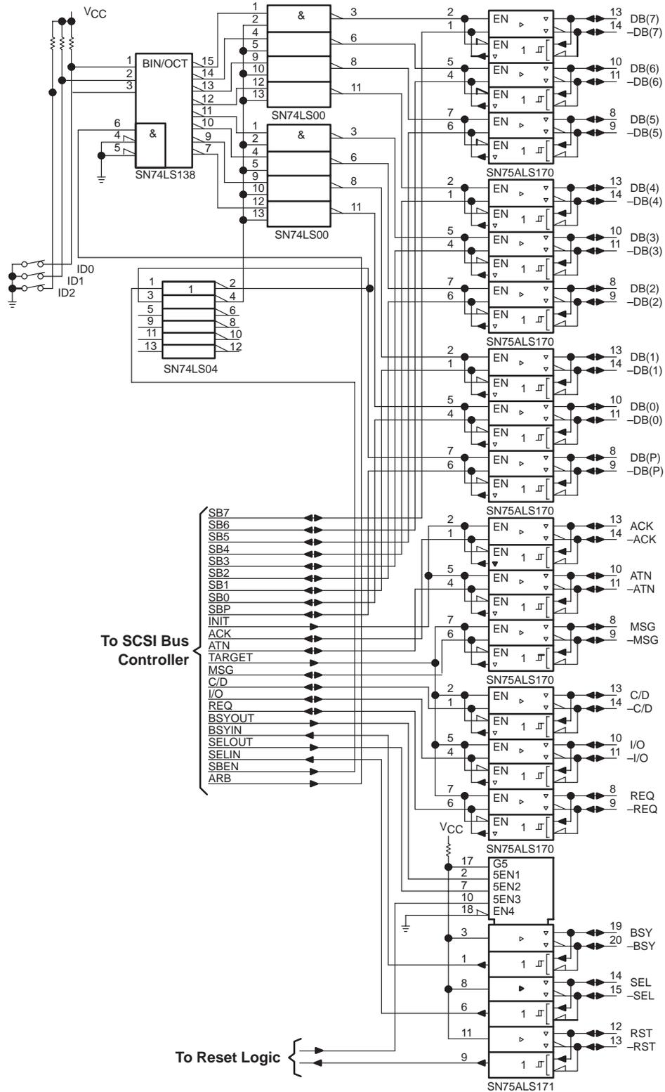
Figure 18. Typical Differential SCSI Bus Interface Implementation
