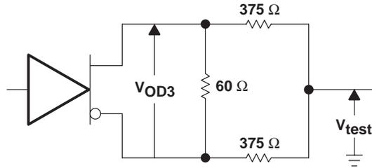
Figure 2. Driver  $V_{OD3}$
