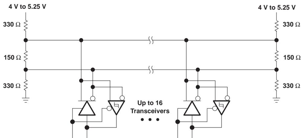
Figure 17. Typical Differential SCSI Application Circuit
