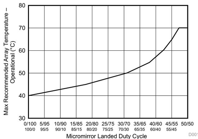
Figure 1. Max Recommended Array Temperature - Derating Curve
