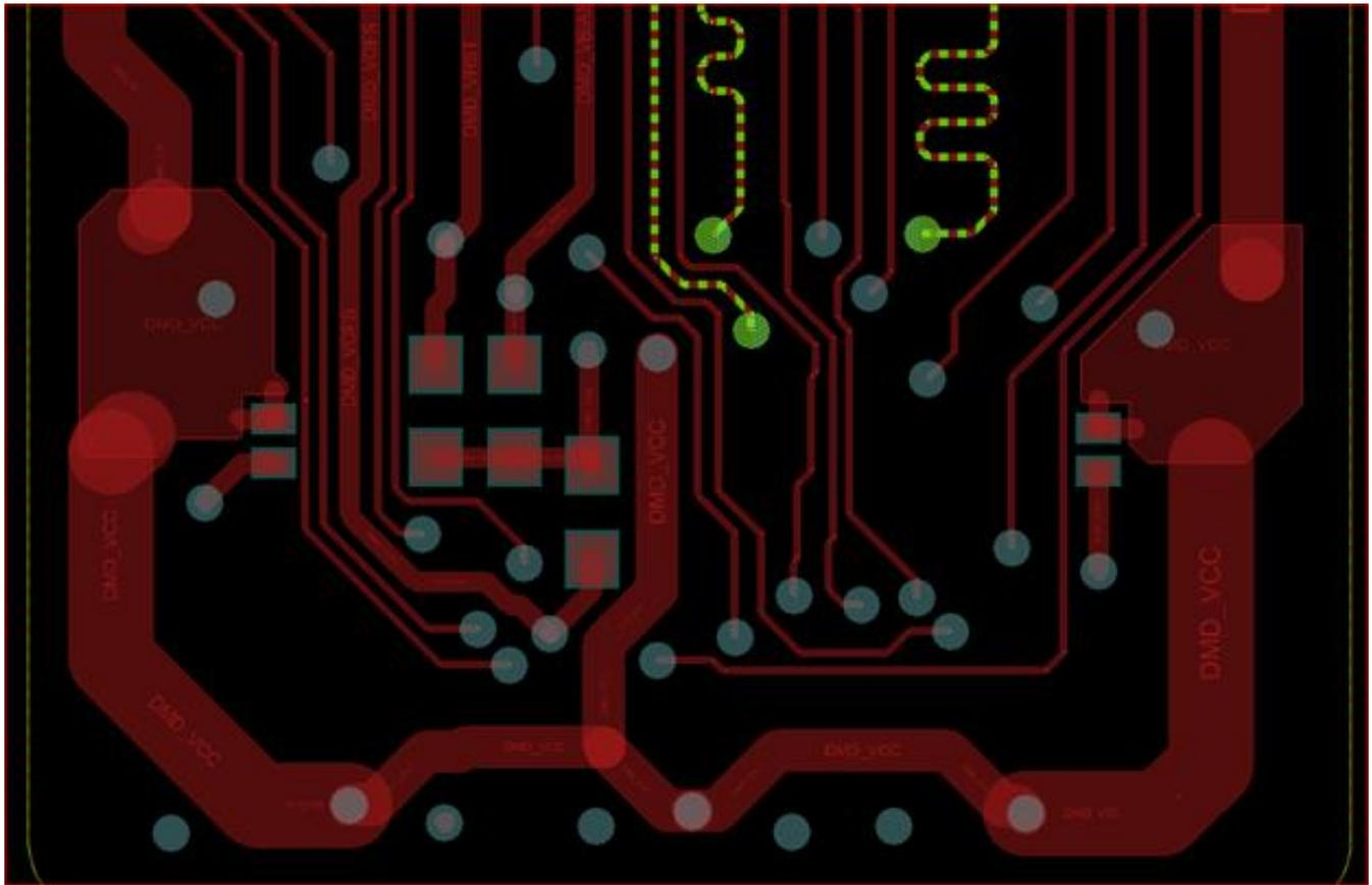
Figure 15. DMD Flex Cable - Bottom Layer
