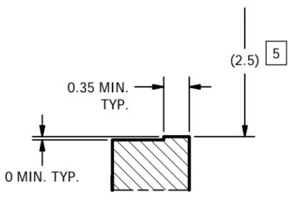
(PANASONIC AXT642124DD1, 42-CONTACT, 0.4 mm PITCH BOARD-TO-BOARD HEADER) INTERFACE TO PANASONIC AXT542124DD1 SOCKET
