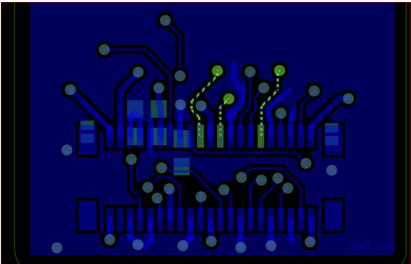
**Figure 14. DMD Flex Cable - Top Layer**
