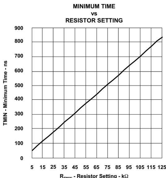
**Figure 12. Minimum Time TMIN Over Setting Resistor R<sub>TMIN</sub>**
