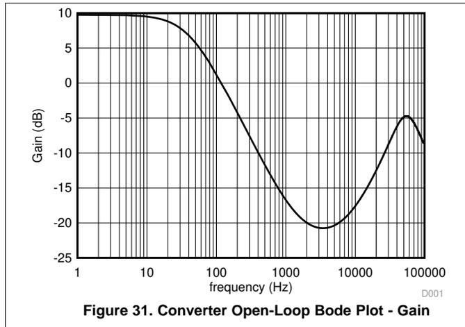
**Figure 31. Converter Open-Loop Bode Plot - Gain**
