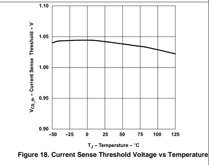
Figure 18. Current Sense Threshold Voltage vs Temperature
