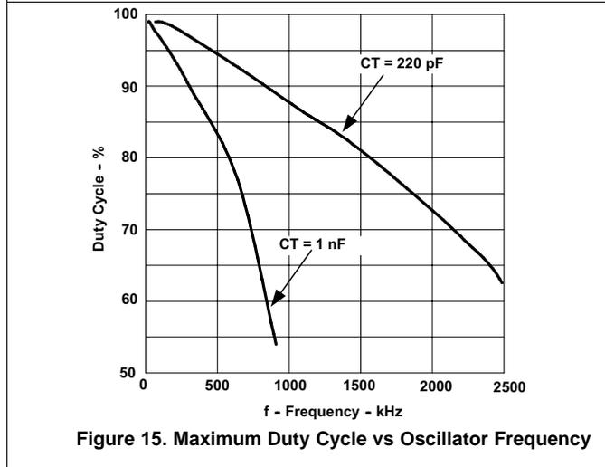
Figure 15. Maximum Duty Cycle vs Oscillator Frequency
