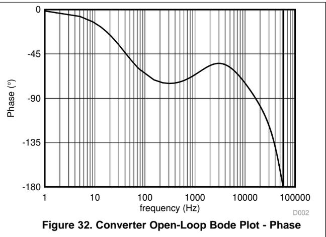
**Figure 32. Converter Open-Loop Bode Plot - Phase**
