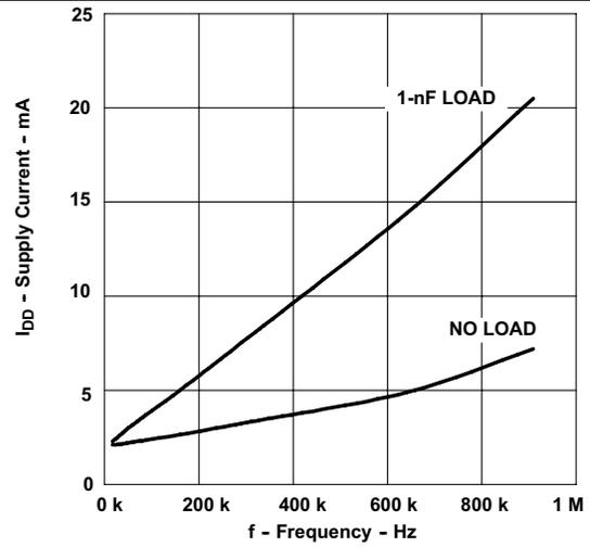
Figure 12. Supply Current vs Oscillator Frequency
