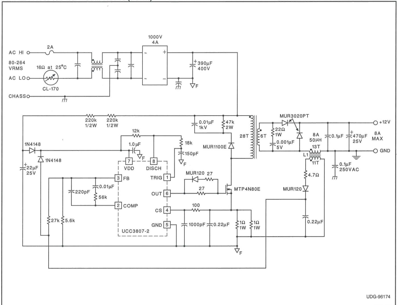
Figure 2. Typical Off-line Application Using UCC3807-2
