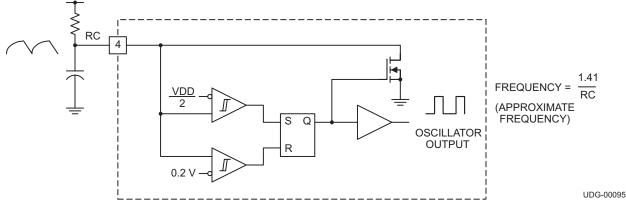
A. The oscillator generates a sawtooth waveform on RC. During the RC rise time, the output stages alternate on time, but both stages are off during the RC fall time. The output stages switch a 1/2 the oscillator frequency, with ensured duty cycle of < 50% for both outputs.
