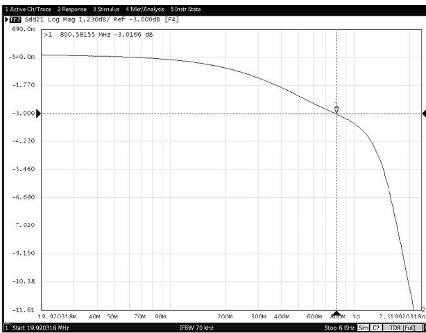
Figure 8-23. Data Transmission Characteristics vs Frequency
