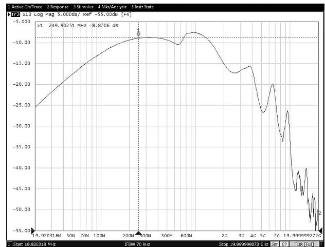
Figure 8-24. Off-State Data-Switch Isolation vs Frequency
