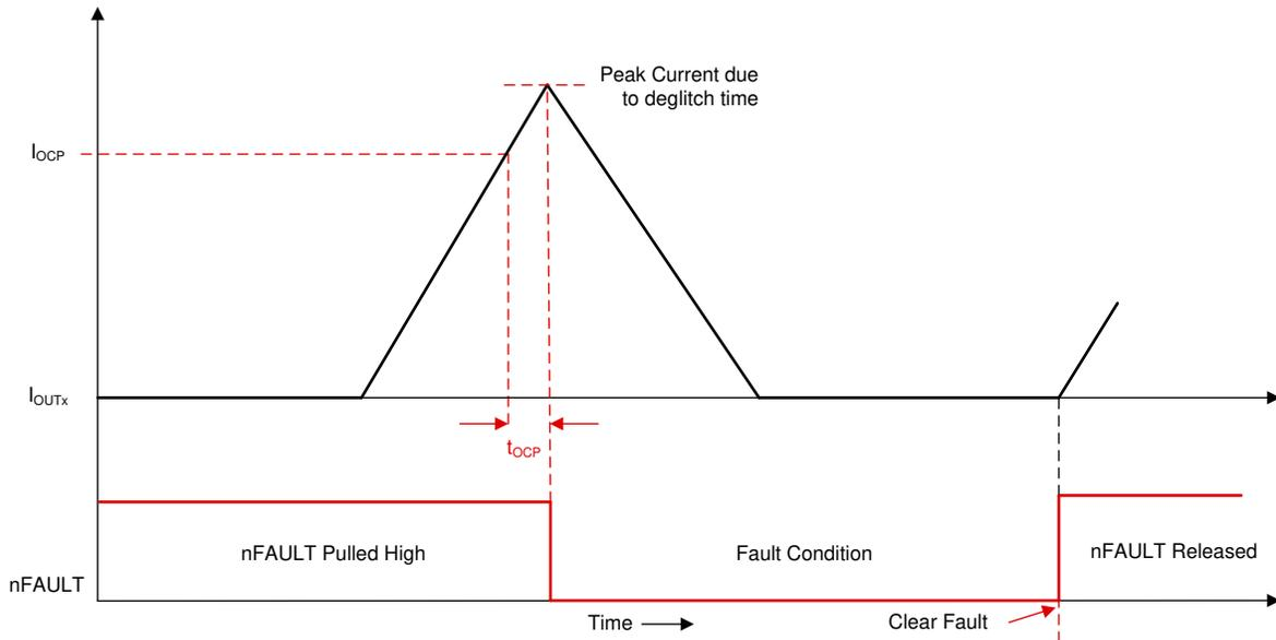
Figure 8-42. Overcurrent Protection - Latched Shutdown Mode
