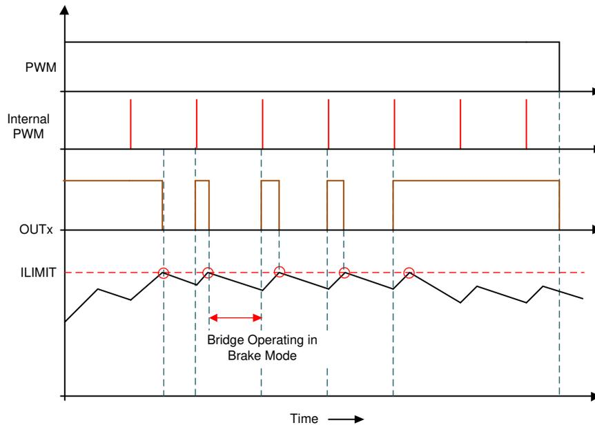
Figure 8-39. Cycle-by-Cycle Current-Limit Operation with 100% PWM Duty Cycle
