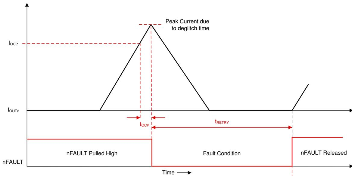
Figure 8-43. Overcurrent Protection - Automatic Retry Mode
