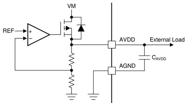
**Figure 8-8. AVDD Linear Regulator Block Diagram**
