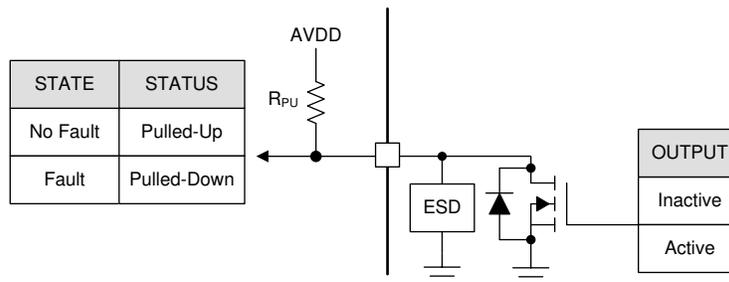
Figure 8-24. Open Drain
