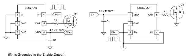
in- is Grounded to the Enable Output)
