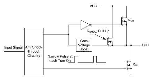
图 23. UCC2751x Gate Driver Output Structure
