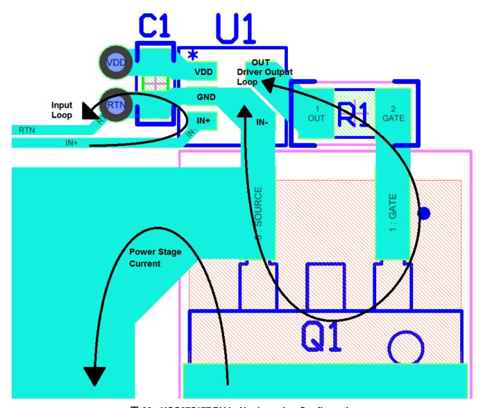
图 29. UCC27517DBV in Noninverting Configuration
