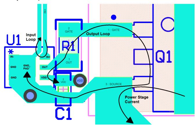
图 28. UCC27516DRS in Noninverting Configuration
