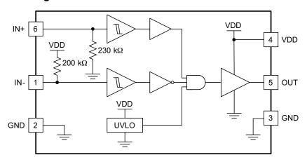
图 19. UCC27516 Functional Block Diagram
