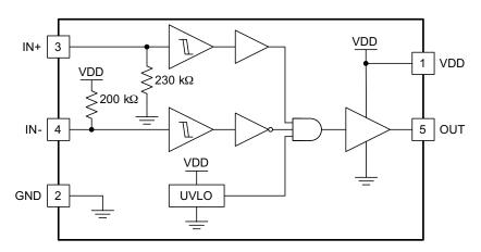
图 20. UCC27517 Functional Block Diagram
