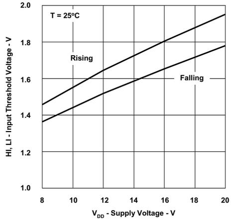
Figure 7. UCC27201A Input Threshold vs Supply Voltage
