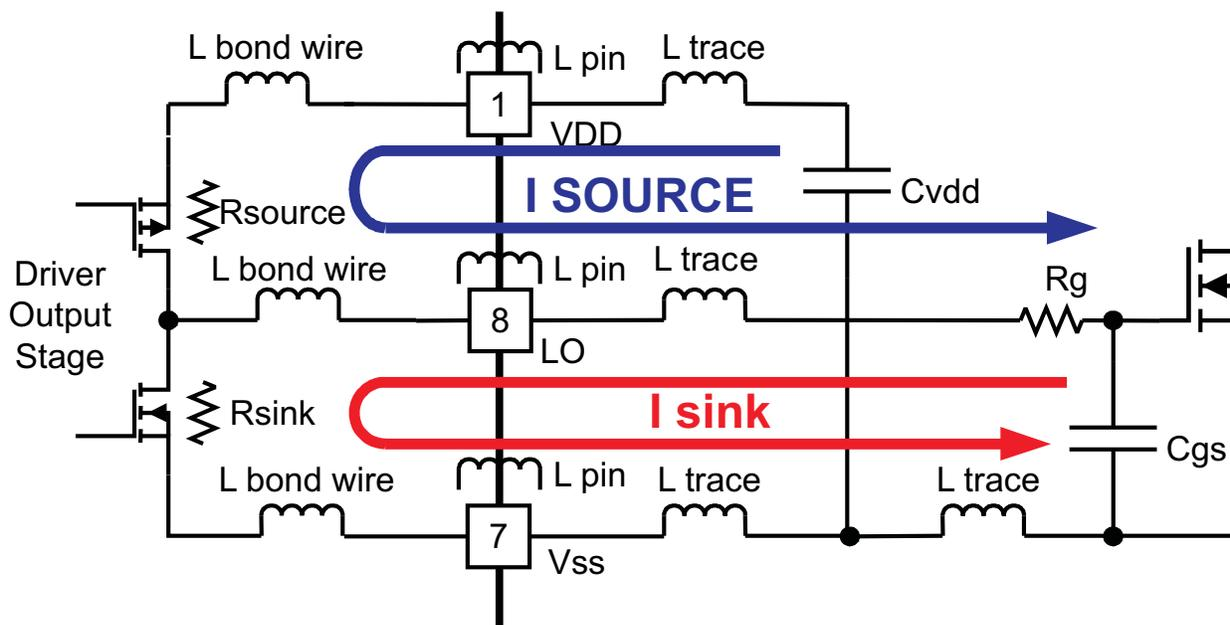
Figure 23. MOSFET Drive Paths and Circuit Parasitics
