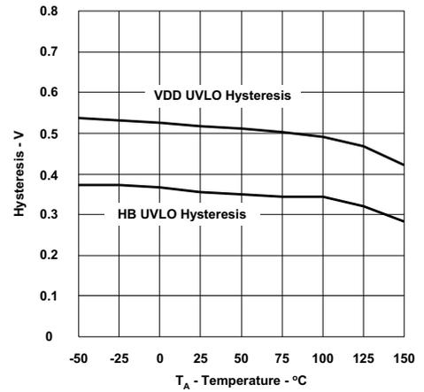
Figure 13. Undervoltage Lockout Threshold Hysteresis vs Temperature
