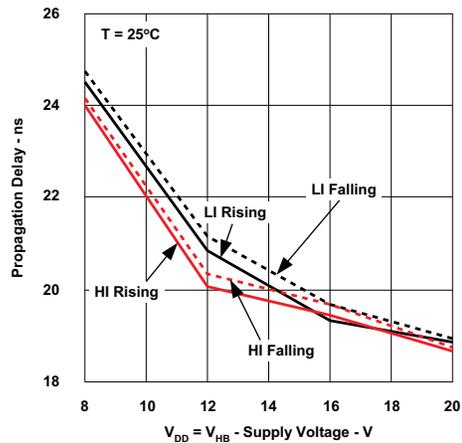
Figure 17. UCC27201A Propagation Delay vs Supply Voltage
