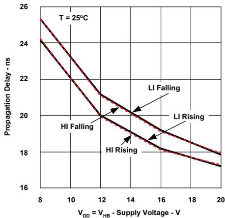
Figure 16. UCC27200A Propagation Delay vs Supply Voltage
