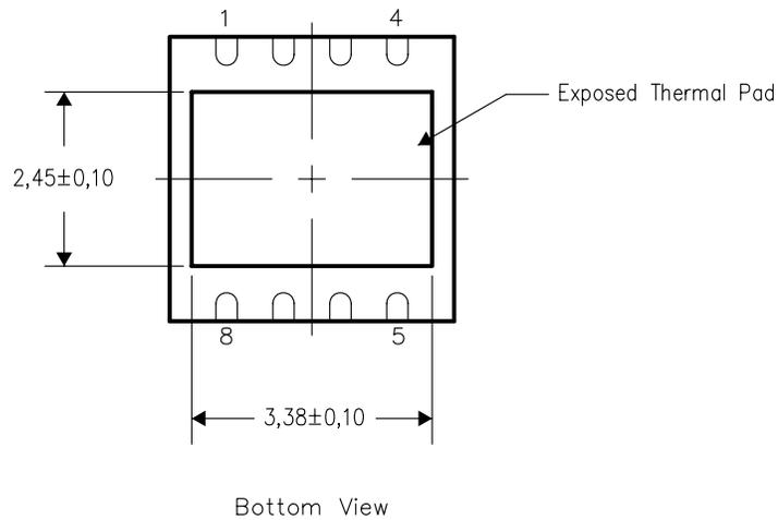
NOTE: All linear dimensions are in millimeters
