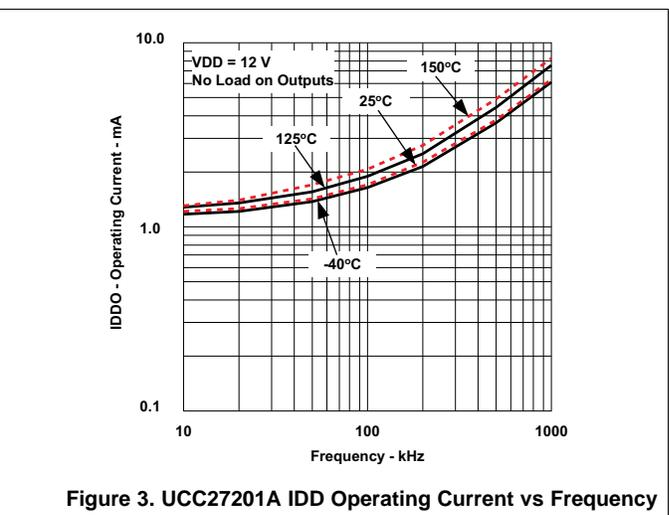
Figure 3. UCC27201A IDD Operating Current vs Frequency
