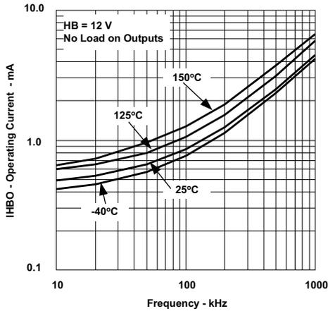
Figure 4. Boot Voltage Operating Current vs Frequency
