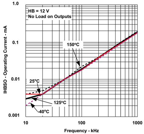
Figure 5. HB to VSS Operating Current vs Frequency
