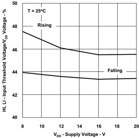
Figure 6. UCC27200A Input Threshold vs Supply Voltage
