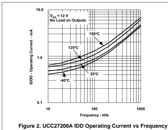
Figure 2. UCC27200A IDD Operating Current vs Frequency
