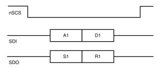
图 33. SPI Transaction Between MCU and the device
