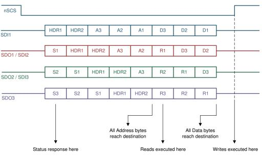
图 36. SPI Frame With Three Devices
