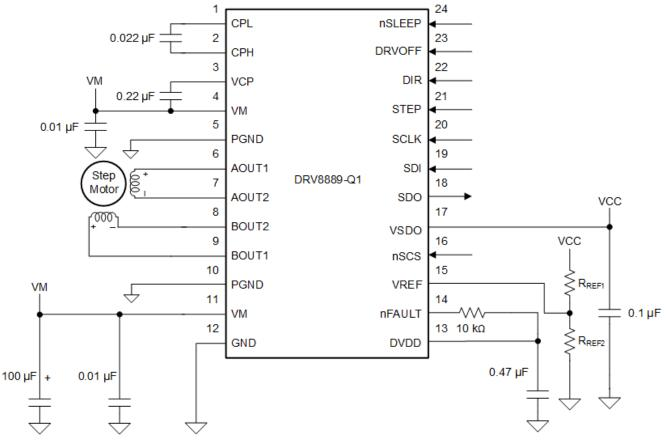
图 52. Typical Application Schematic (HTSSOP package)
