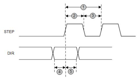
图 1. STEP and DIR Timing Diagram
