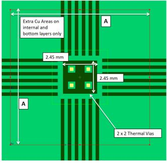
图 63. PCB - Top Layer (4/2-Layer PCB) for VQFN Package
