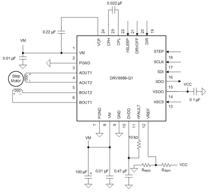
图 53. Typical Application Schematic (VQFN package)
