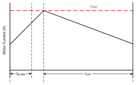
图 15. Current Chopping Waveform
