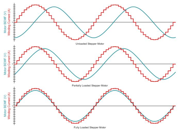
图 31. Stall Detection by Monitoring Motor Back-EMF
