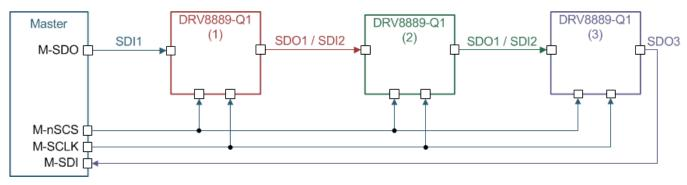
图 35. Three DRV8889-Q1 Devices Connected in Daisy Chain
