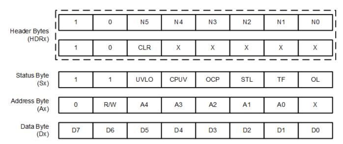
图 39. Contents of Header, Status, Address, and Data Bytes for DRV8889-Q1
