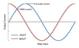
图 11. Full-Scale and RMS Current
