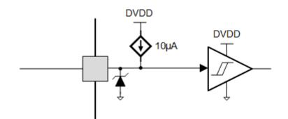
图 27. Logic-Level with Internal Pull-up Input Pin Diagram
