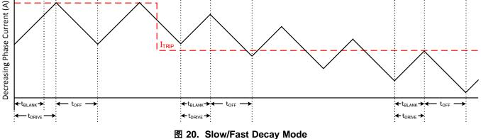
During fast decay, the polarity of the H-bridge is reversed. The H-bridge will be turned off as current approaches zero in order to prevent current flow in the reverse direction. In this mode, fast decay only occurs during decreasing current. Slow decay is used for increasing current.
