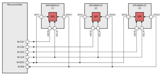
图 34. Three DRV8889-Q1 Devices Connected in Parallel Configuration
