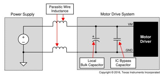
图 72. Example Setup of Motor Drive System With External Power Supply
