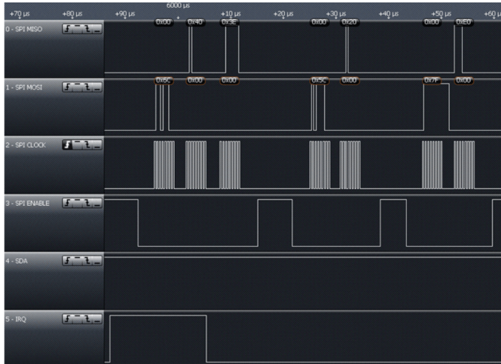
Figure 6-24. IRQ With One Byte in FIFO
