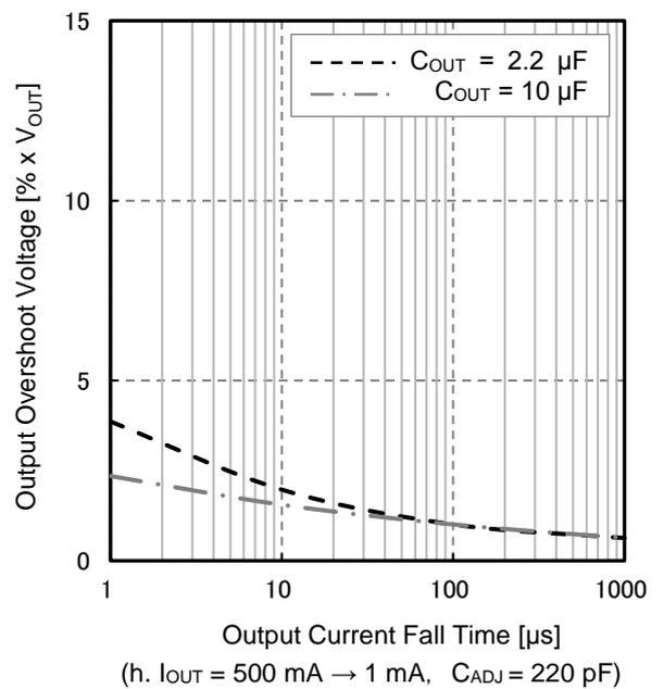
Figure 19. Load Transient Response
