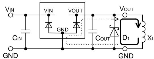
Figure 33. Current Path in Inductive Load (Output: Off)
