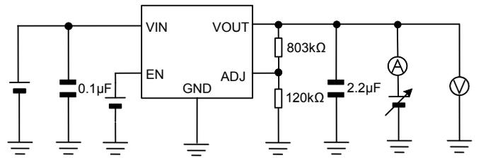
Measurement Setup for Figure 7
