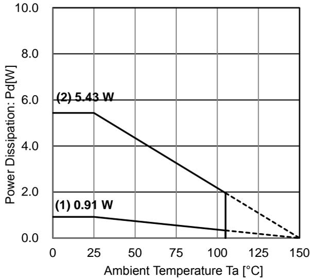
Figure 34. Power Dissipation Graph (TO252-5)
