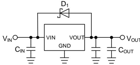
Figure 27. Bypass Diode for Reverse Current Diversion
