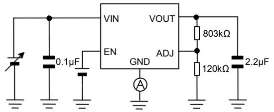
Measurement Setup for Figure 4, 5, 8, 22
