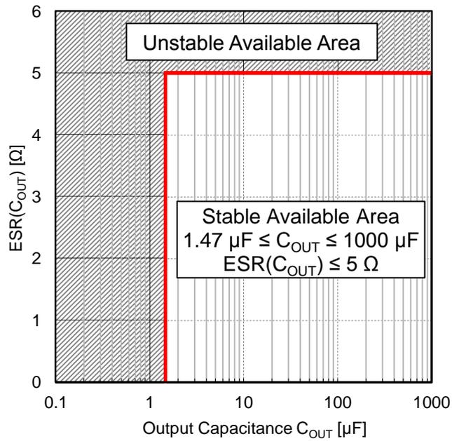
Figure 23. Output Capacitance C<sub>OUT</sub>, ESR Stable Available Area
