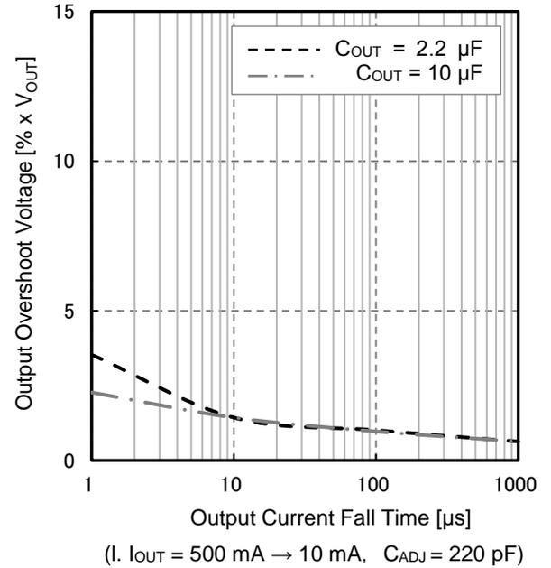
Figure 20. Load Transient Response
