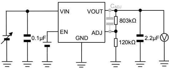
Measurement Setup for Figure 1, 2, 3, 10, 15, 17, 18
