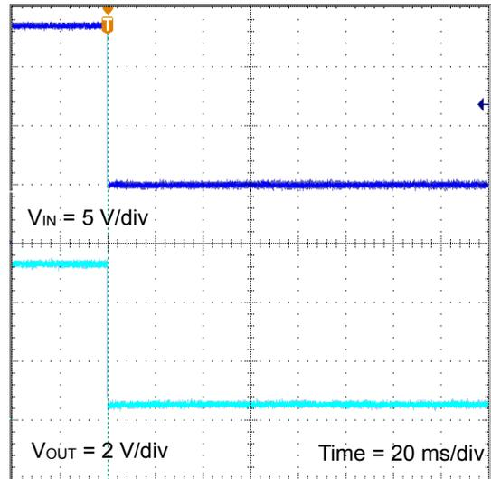
(h.  $V_{IN} = 13.5\text{ V} \rightarrow 0\text{ V}$ ,  $C_{OUT} = 10\text{ }\mu\text{F}$ )
