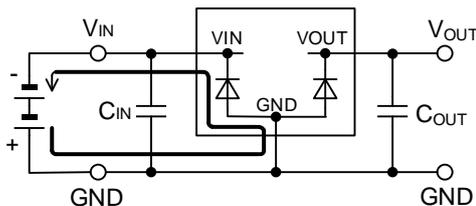
Figure 29. Current Path in Reverse Input Connection
