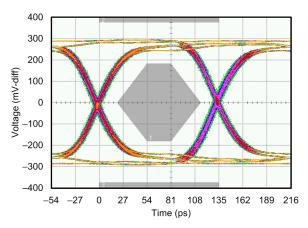
Figure 36. Output Serial Lane Eye Diagram at 7.4Gb/s
