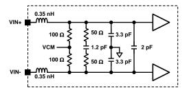
Figure 55. Simplified Analog Input Network Circuit Model
