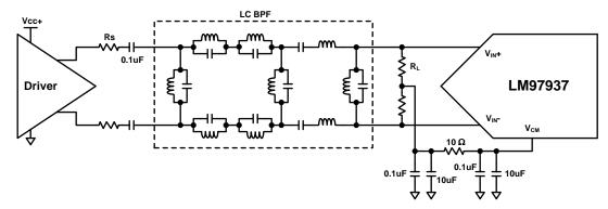
Figure 59. Bandpass Filter Anti-Aliasing Interface
