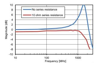
Figure 57. Measured Input Voltage Frequency Response
