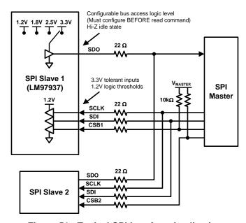
Figure 51. Typical SPI Interface Application
