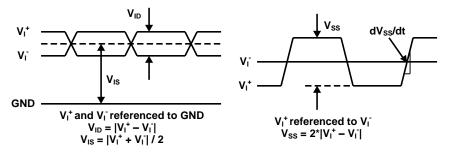
Figure 4. Electrical Level Diagram for Differential Input Signals
