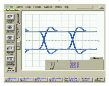
Figure 45. De-Emphasis of the Differential Output Signal
