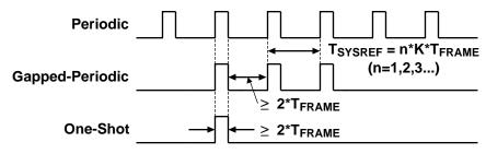
Figure 67. SYSREF Signal Types (Single-Ended Representations)
