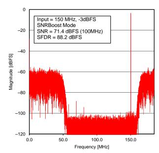
Figure 1. 1-Tone Spectrum, SNRBoost Mode, 150 MHz
