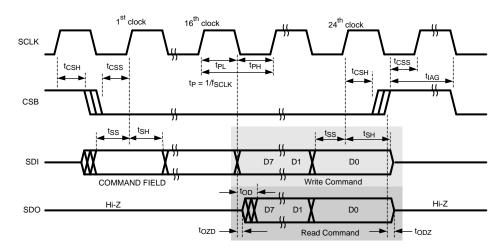
Figure 10. SPI Timing Diagram
