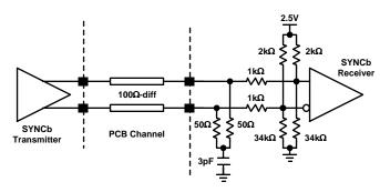
Figure 68. SYNCb Input Receiver and Interface
