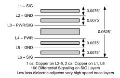
Figure 70. Recommended PCB Layer Stack-Up for a 6-Layer Board
