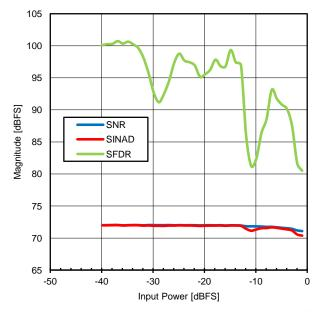
Figure 13. SNR, SINAD, SFDR vs. Input Frequency
