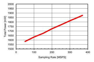
Figure 34. Power vs. Sampling Rate
