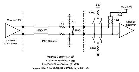
Figure 66. Example DC Coupling to the SYSREF Input
