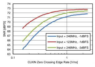
Figure 64. SNR vs. Input Clock Edge Rate
