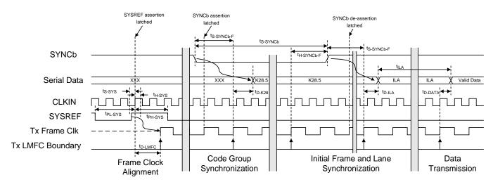
Figure 49. Link Initialization Timing and Flow Diagram
