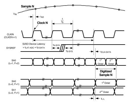
Figure 9. Sample to Data Timing Diagram
