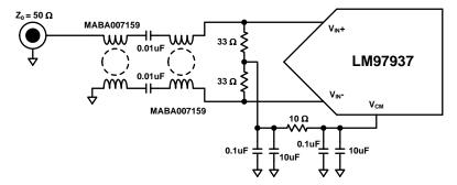
Figure 58. Transformer Input Network
