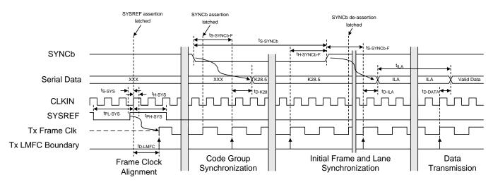
Figure 12. JESD204B Interface Link Initialization Timing Diagram
