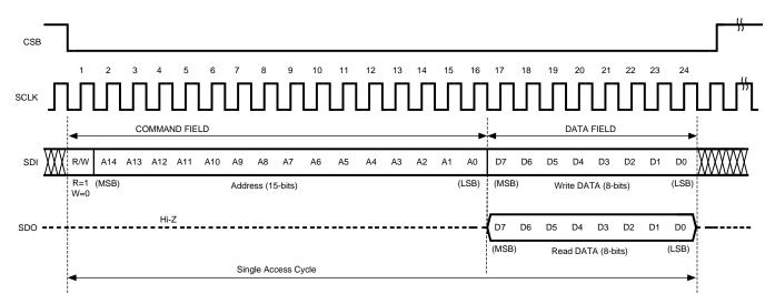
Figure 52. Serial Interface Protocol
