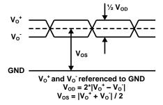
Figure 6. Electrical Level Diagram for Differential Output Signals
