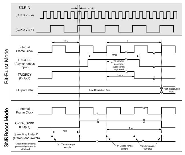
Figure 11. Trigger and Over-Range Timing Diagrams
