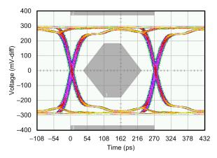
Figure 37. Output Serial Lane Eye Diagram at 3.7Gb/s
