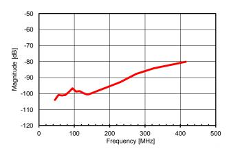
Figure 32. Crosstalk vs. Input Frequency
