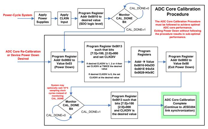
Figure 46. Device Start-Up Flow Chart
