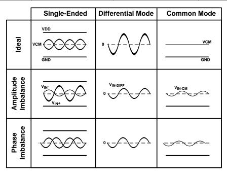
Figure 54. Differential Signal Waveform and Signal Imbalance
