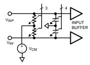
Figure 43. Simplified Input Differential Balance Correction Circuit
