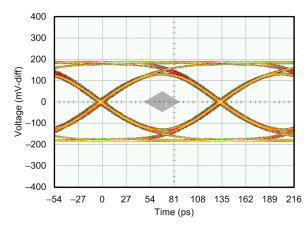
Figure 38. Transmitted Eye at Output of 20in. 5 mil. FR4 Microstrip at 7.4Gb/s with Optimized De-Emphasis
