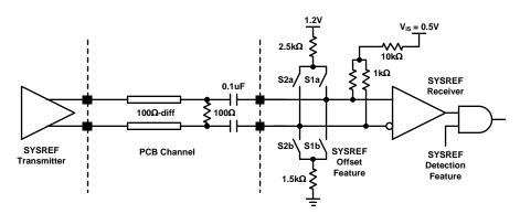
Figure 65. SYSREF Input Receiver and AC Coupled Interface
