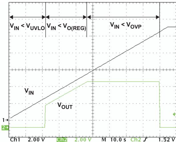
Figure 6. OUT Pin Response to Slow Input Ramp
