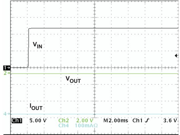
Figure 3. Power-On with Input Overtolerance.
