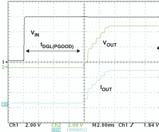
Figure 2. Normal Power-On Showing Soft-Start.
