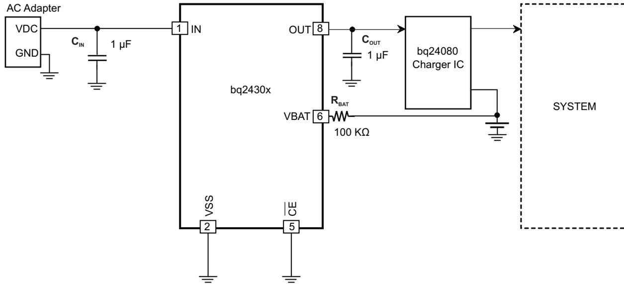
Figure 22. Overvoltage, Overcurrent, and Battery Overvoltage Protection
