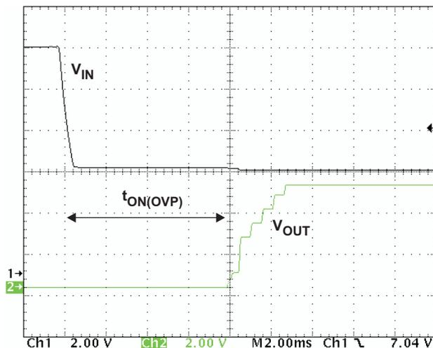
Figure 7. bq24300 Recovery from Input OVP.
