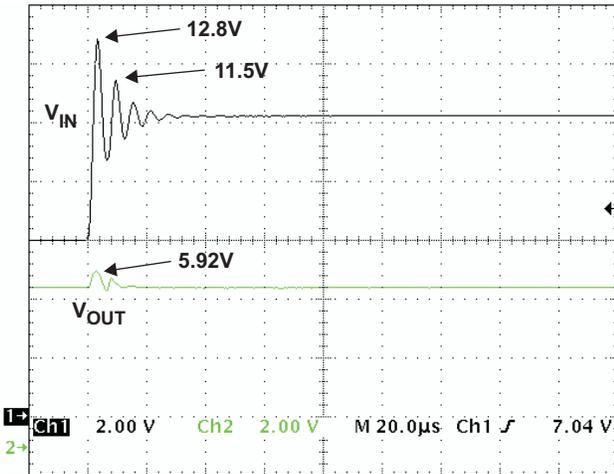
Figure 4. bq24300 OVP Response for Input Step.
