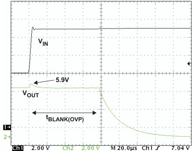
Figure 5. bq24300 OVP Response for Input Step.
