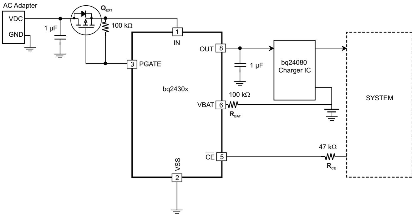
Figure 23. OVP, OCP, BATOV With Input Reverse-Polarity Protection
