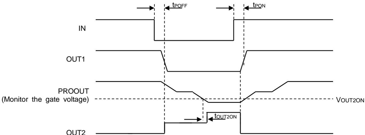
Figure 5. Timing chart of Miller Clamp function
