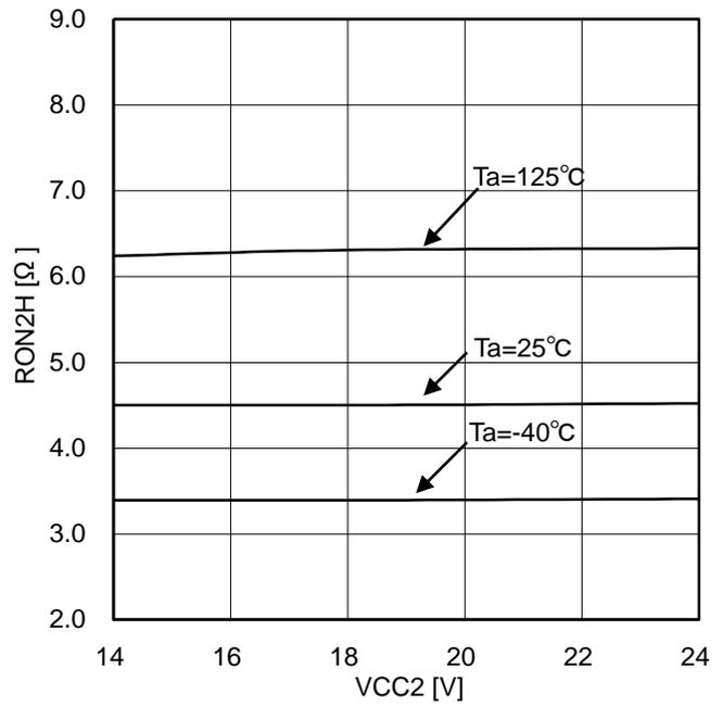
Figure 44. OUT2 ON resistance (Source)
