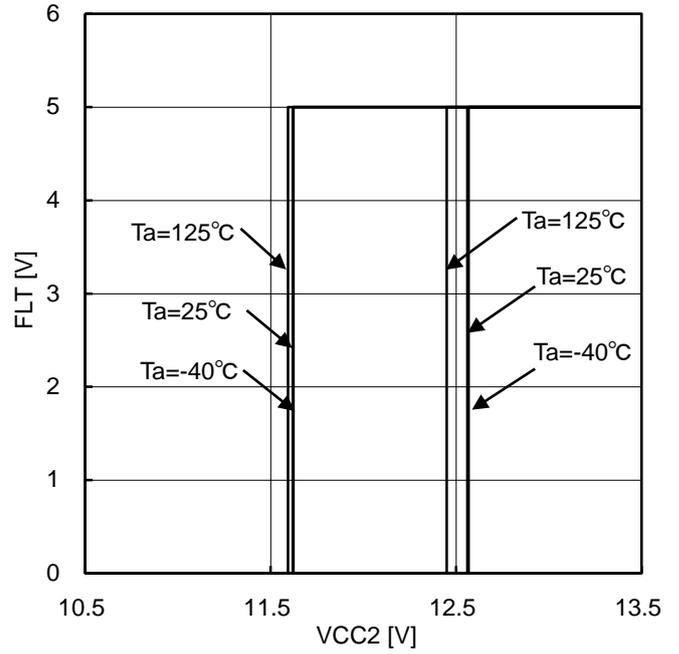
Figure 52. VCC2 UVLO ON/OFF voltage (at VCC1=5V)
