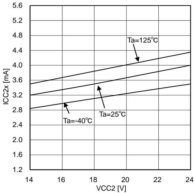
Figure 25. Output side circuit current (at OUT1=L)
