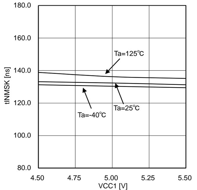
Figure 34. Logic (INA/INB) input mask time (Low pulse)
