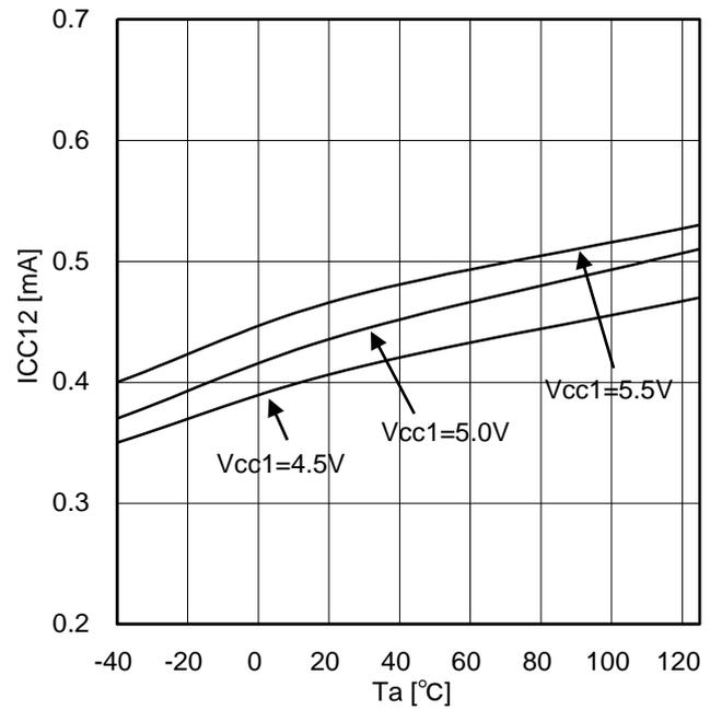
Figure 20. Input side circuit current (at OUT1=H)
