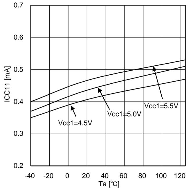
Figure 18. Input side circuit current (at OUT1=L)
