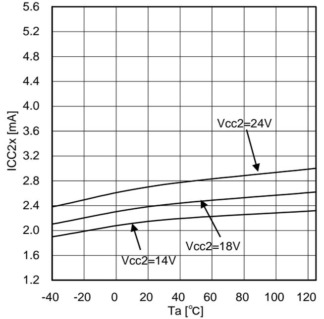
Figure 28. Output side circuit current (at OUT1=H)
