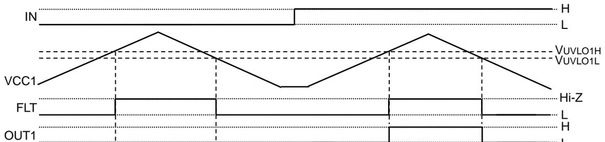
Figure 8. Input-side UVLO Function Operation Timing Chart
