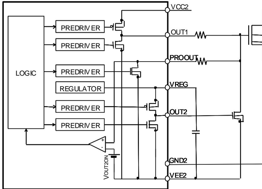
Figure 4. Block diagram of Miller Clamp function
