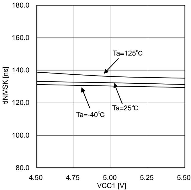
Figure 33. Logic (INA/INB) input mask time (High pulse)
