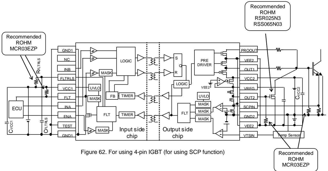
Figure 62. For using 4-pin IGBT (for using SCP function)
