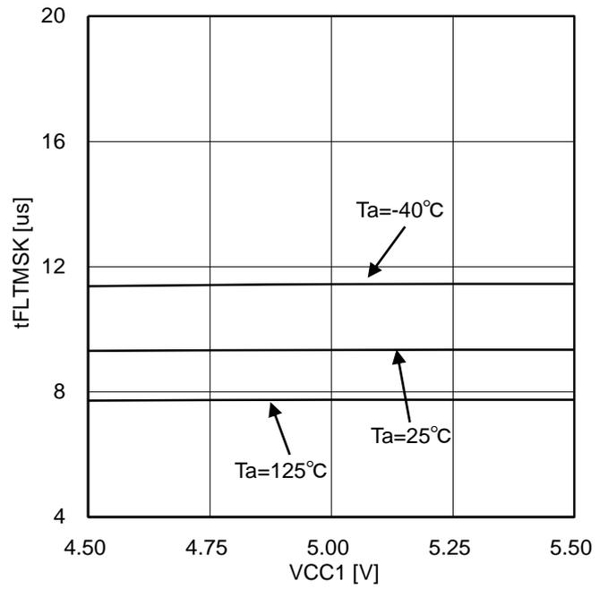
Figure 36. FLT input mask time
