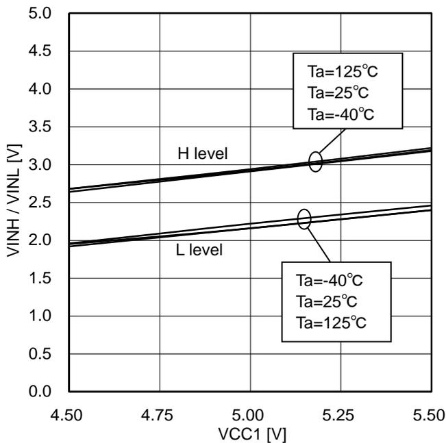
Figure 29. Logic (INA/INB/ENA) High/Low level input voltage
