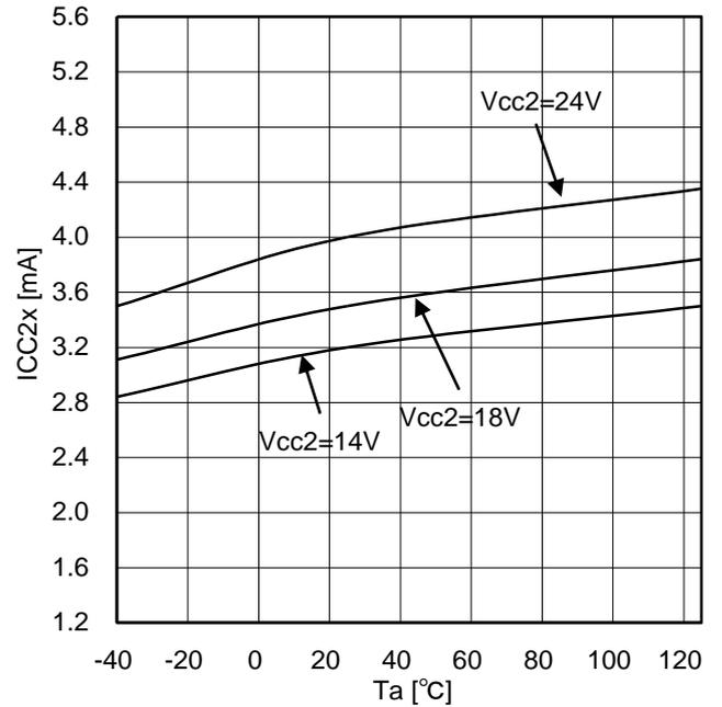
Figure 26. Output side circuit current (at OUT1=L)
