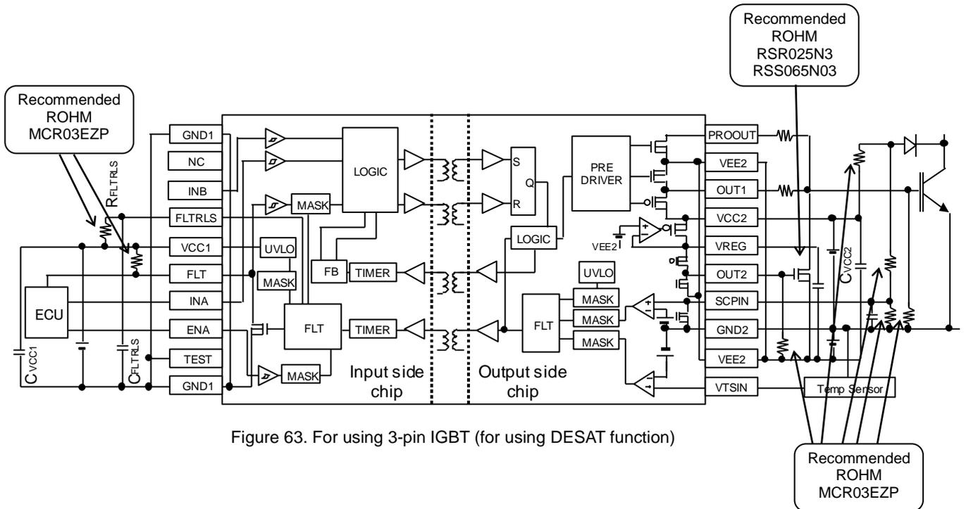
Figure 63. For using 3-pin IGBT (for using DESAT function)
