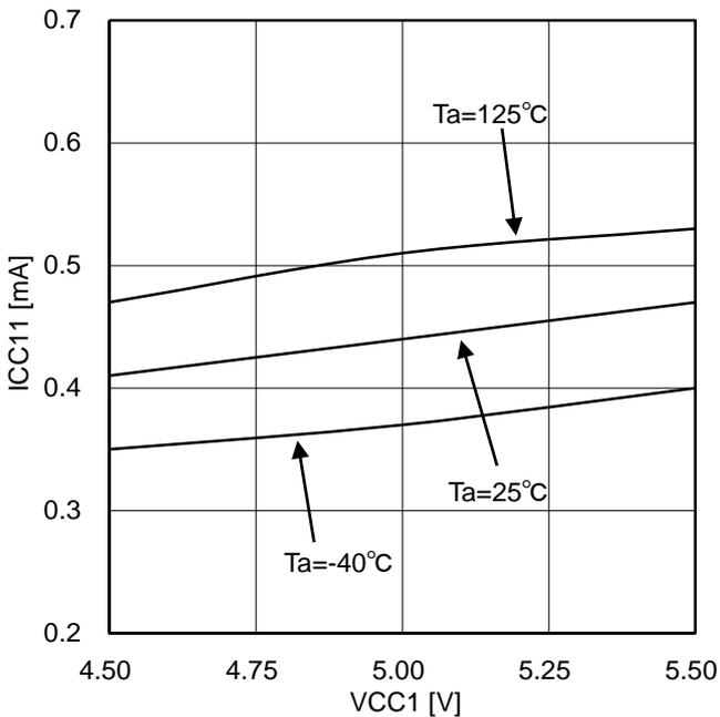
Figure 17. Input side circuit current (at OUT1=L)
