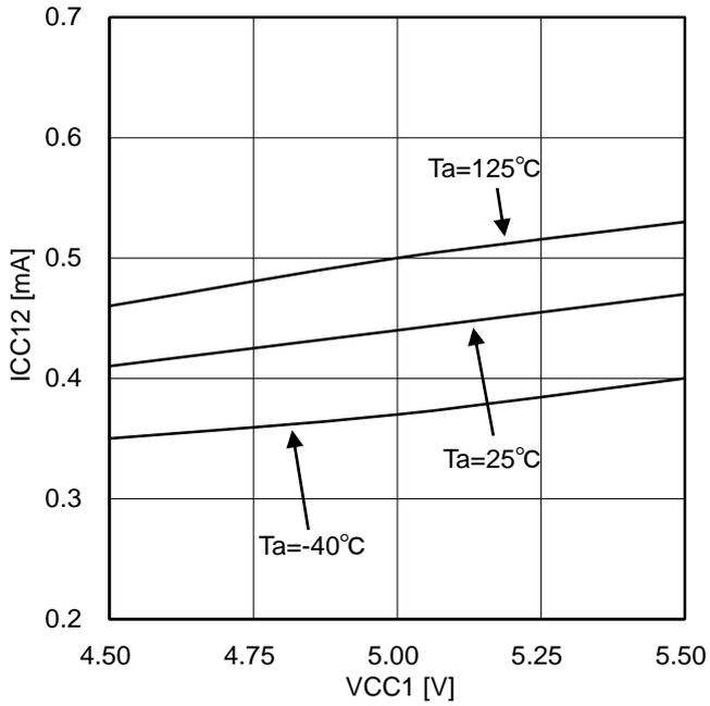
Figure 19. Input side circuit current (at OUT1=H)
