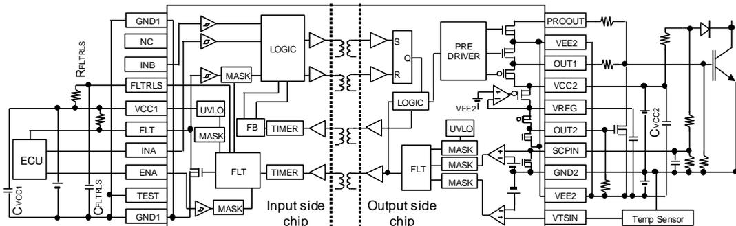
Figure 2. For using 3-pin IGBT (for using DESAT function)
