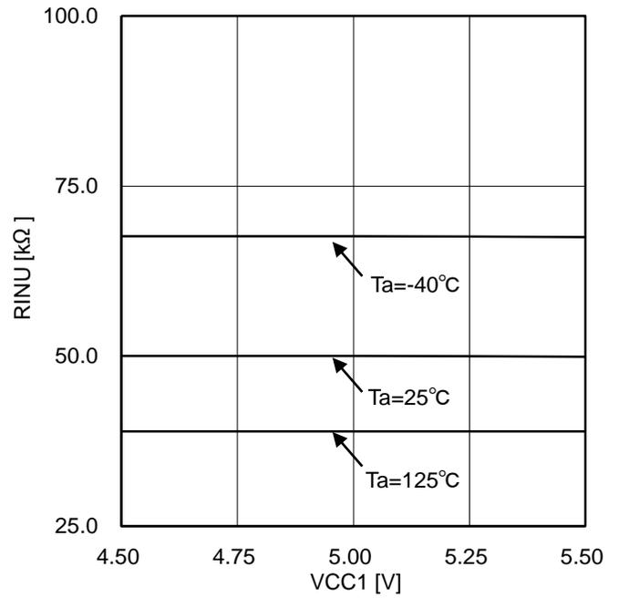
Figure 32. Logic pull-up resistance
