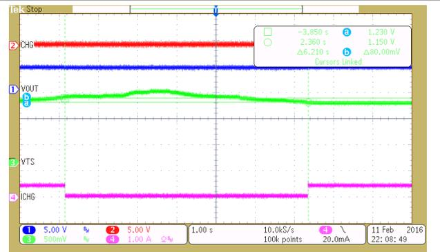
Figure 14. TS Entering and Leaving Cold Temperature
