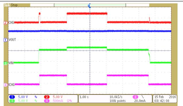
Figure 16. OVP From Normal Power-Up Operation –  $V_{IN} 0V \rightarrow 6V \rightarrow 7V \rightarrow 6V \rightarrow 0V$
