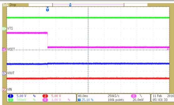
Figure 19. Battery Removal – GND Removed 1st, 42-Ω Load
