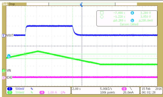
V<sub>IN</sub> swept from 5 V to 3.9 V to 5 V
