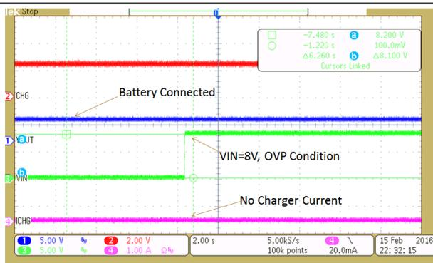
Figure 15. OVP 8-V Adaptor — Hot Plug
