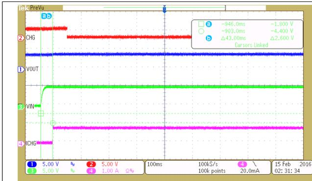
Figure 11. Power-Up Timing
