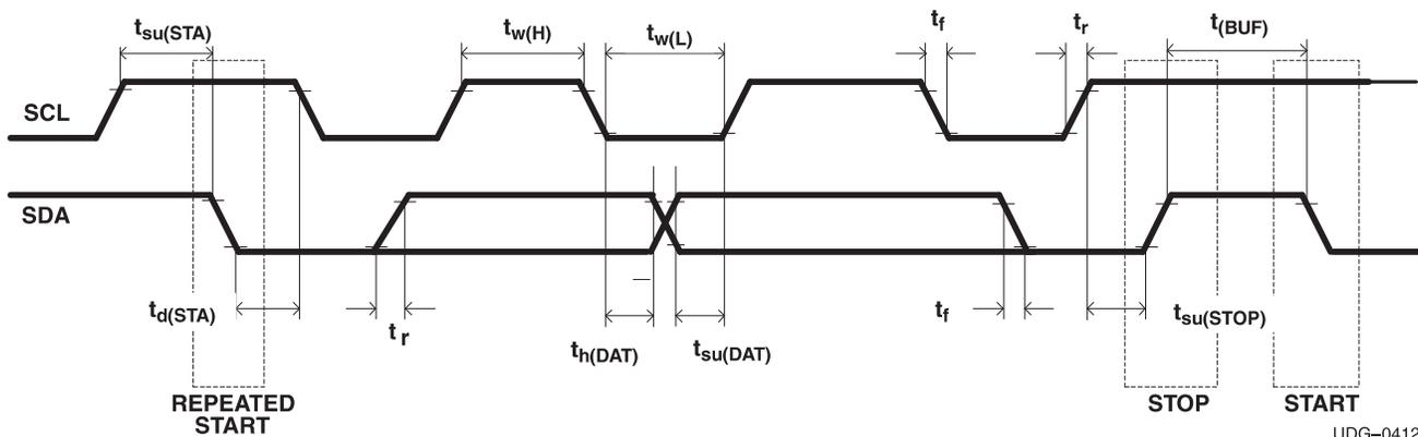
Figure 3-1. I<sup>2</sup>C-Compatible Interface Timing Diagrams
