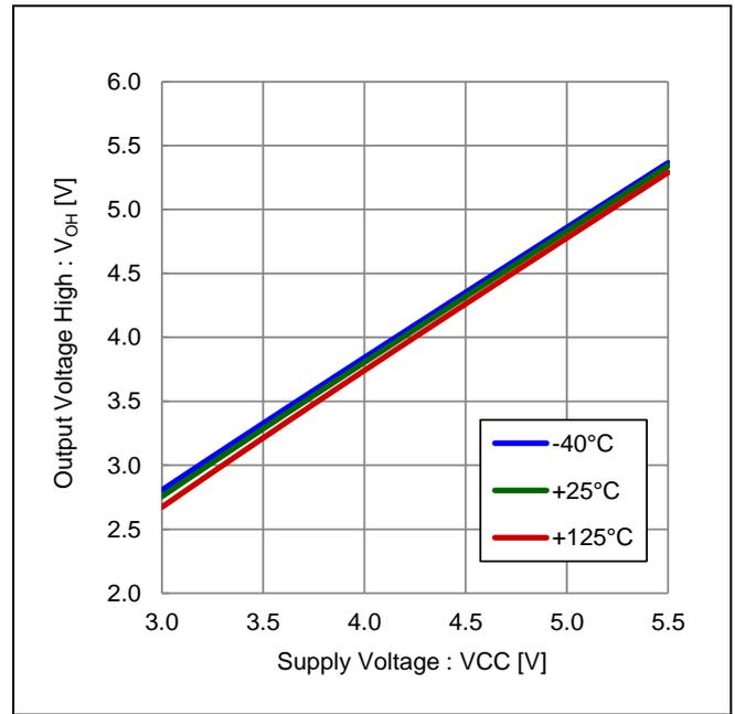
Figure 13. Output Voltage vs Supply Voltage (@I<sub>So</sub>=-4mA)
