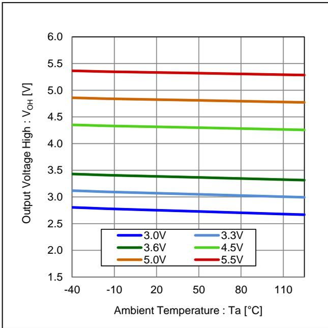
Figure 14. Output Voltage vs Ambient Temperature (@I<sub>So</sub>=-4mA)
