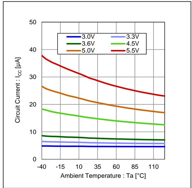
Figure 9. Circuit Current vs Ambient Temperature
