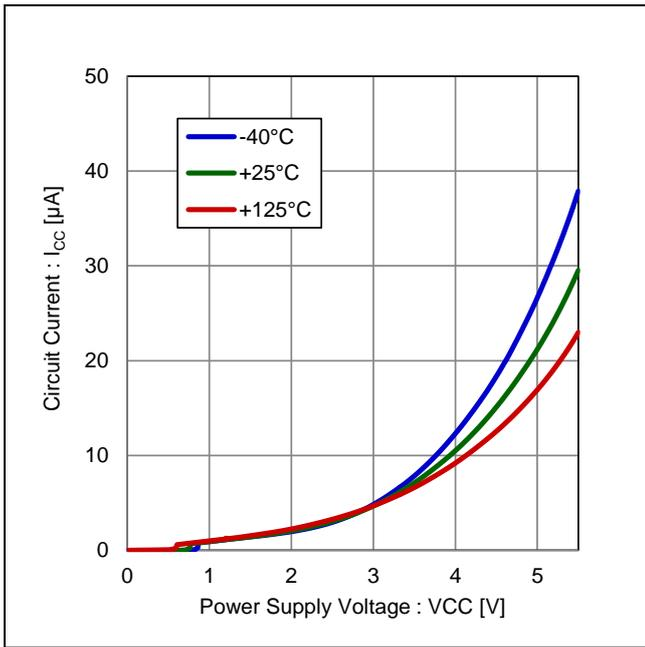
Figure 8. Circuit Current vs Power Supply Voltage
