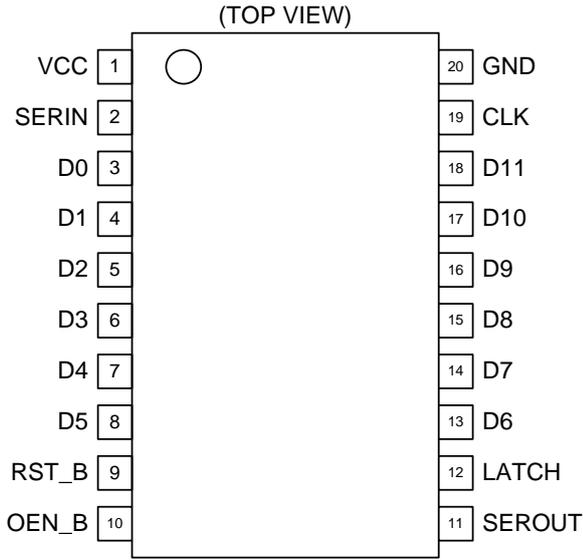
Figure 2. Pin Configuration
