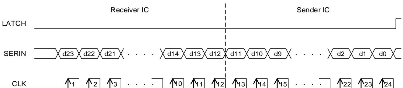
Figure 7. Cascade Connection
