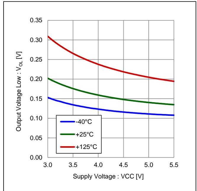
Figure 15. Output Voltage vs Supply Voltage (@I<sub>So</sub>=4mA)
