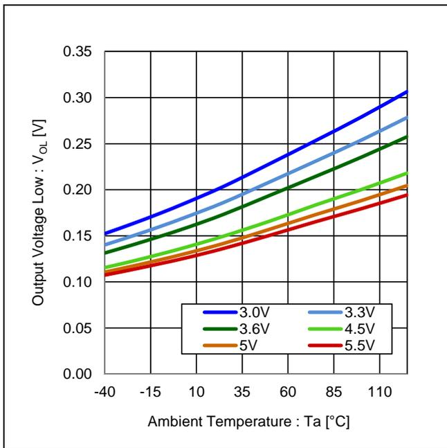
Figure 16. Output Voltage vs Ambient Temperature (@I<sub>SO</sub>=4mA)
