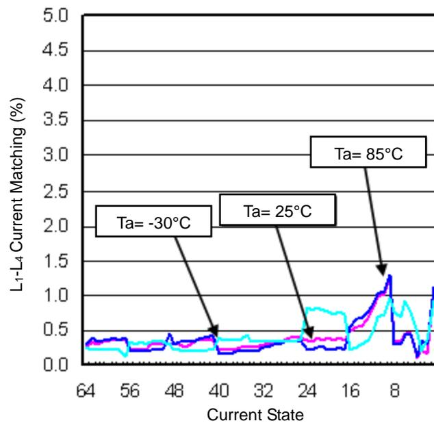
Figure 8. LED Current Relative Accuracy (V<sub>IN</sub> = 3.6 V)
