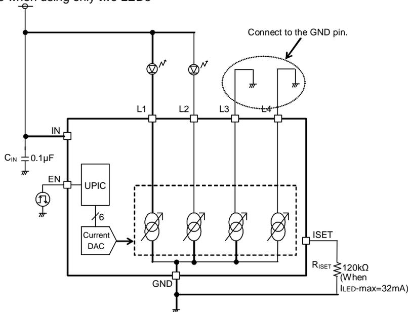
Figure 14. Circuit Example when using only Two LED's
