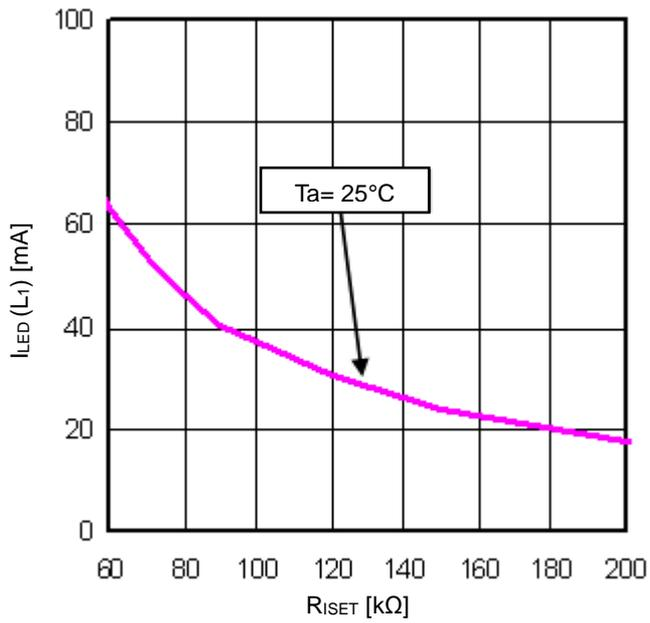
Figure 9. LED Current vs  $R_{ISET}$
