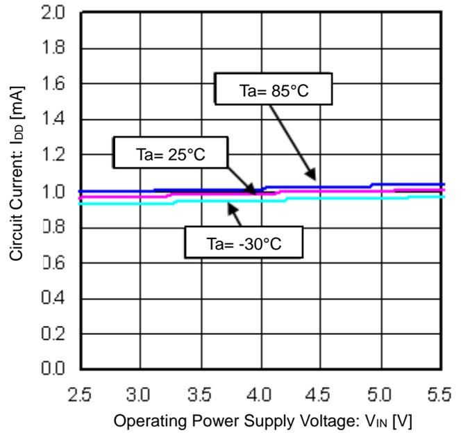
Figure 2. Circuit Current vs Operating Power Supply Voltage
