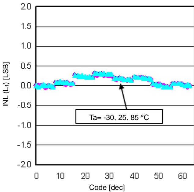
Figure 7. LED Current Characteristics (V<sub>IN</sub> = 3.6 V, Integral Linearity Error)
