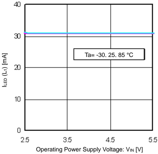
Figure 5. LED Output Current vs Operating Power Supply Voltage (V<sub>IN</sub> = 3.6 V, at 32 mA of LED Current)
