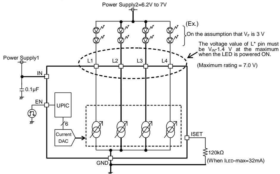
Figure 19. Circuit example when connecting the two LEDs to each of the channels in series
