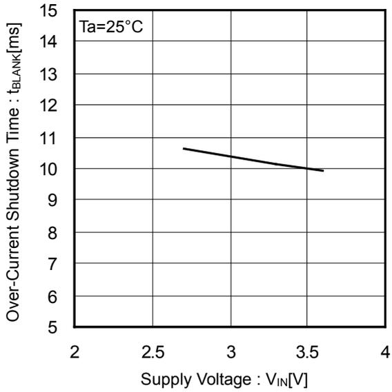
Figure 16. Over-Current Shutdown Time vs Supply Voltage
