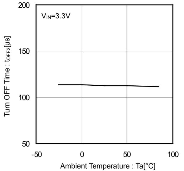
Figure 25. Output Turn OFF Time vs Ambient Temperature
