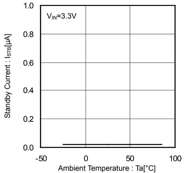
Figure 7. Standby Current vs Ambient Temperature (EN Disable)
