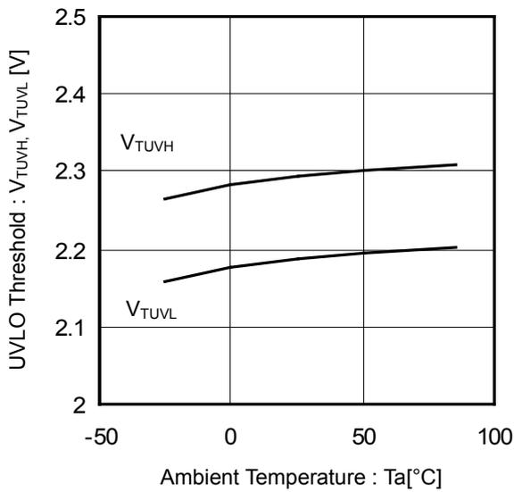
Figure 26. UVLO Threshold Voltage vs Ambient Temperature
