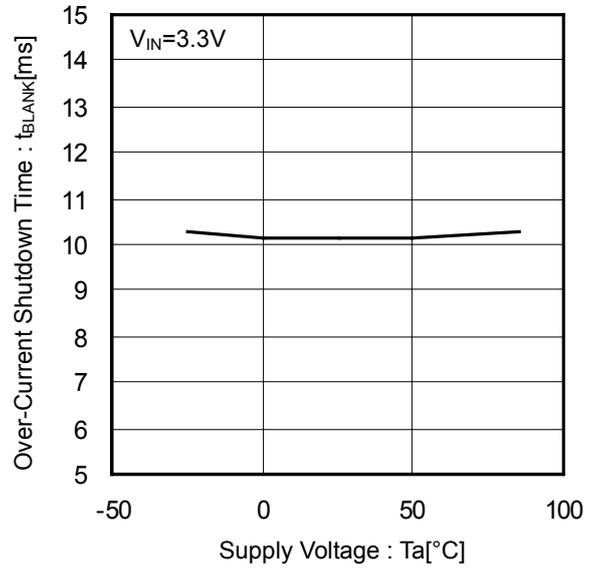
Figure 17. Over-Current Shutdown Time vs Supply Voltage
