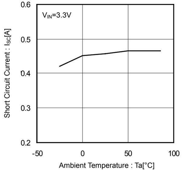
Figure 13. Short Circuit Current vs Ambient Temperature (BD2202G)
