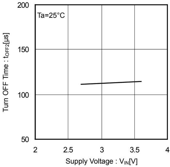
Figure 24. Output Turn OFF Time vs Supply Voltage
