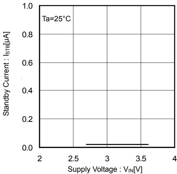
Figure 6. Standby Current vs Supply Voltage (EN Disable)
