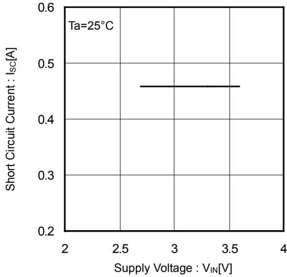
Figure 12. Short Circuit Current vs Supply Voltage (BD2202G)
