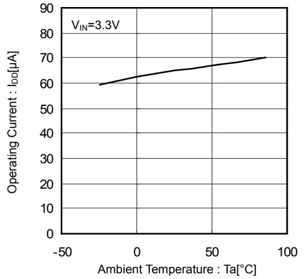
Figure 5. Operating Current vs Ambient Temperature (EN Enable)
