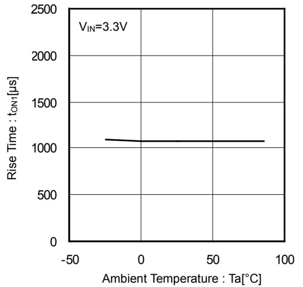
Figure 19. Output Rise Time vs Ambient Temperature
