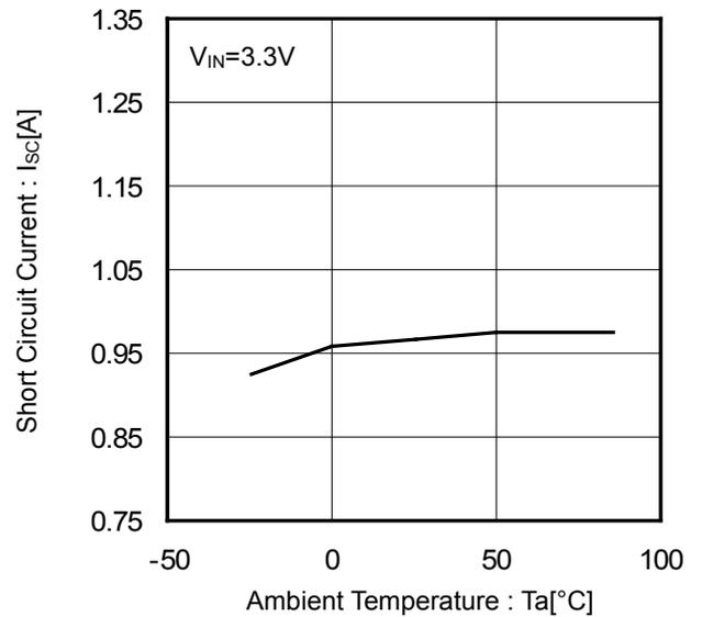
Figure 15. Short Circuit Current vs Ambient Temperature (BD2206G)
