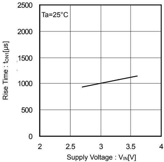
Figure 18. Output Rise Time vs Supply Voltage
