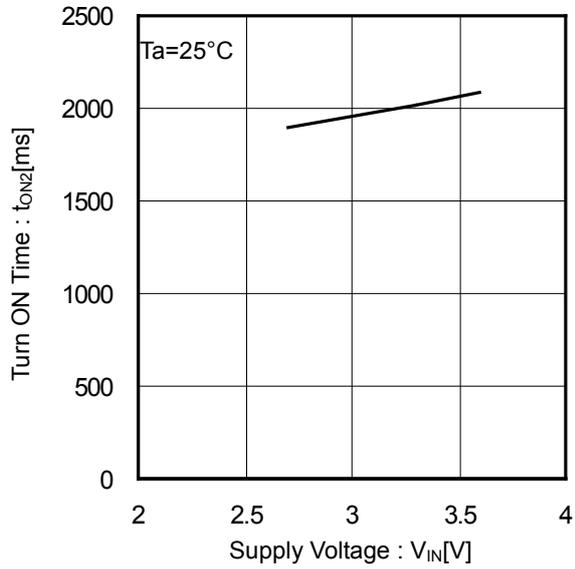
Figure 20. Output Turn ON Time vs Supply Voltage
