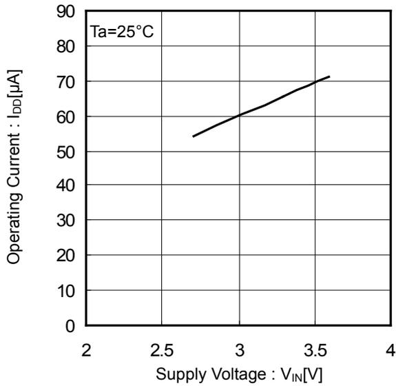
Figure 4. Operating Current vs Supply Voltage (EN Enable)
