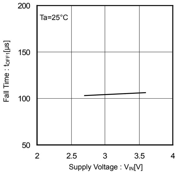
Figure 22. Output Fall Time vs Supply Voltage
