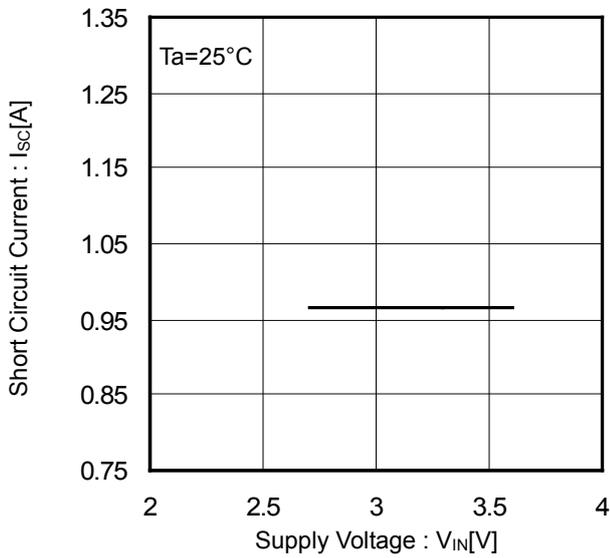
Figure 14. Short Circuit Current vs Supply Voltage (BD2206G)
