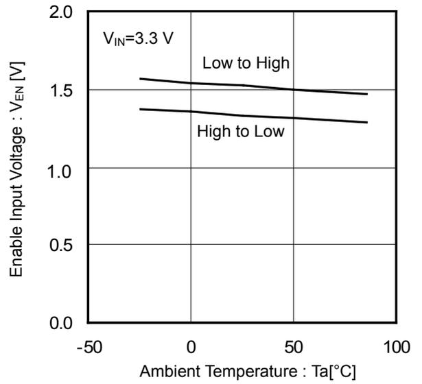
Figure 9. EN Input Voltage vs Ambient Temperature
