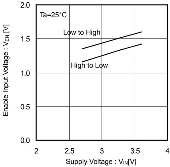
Figure 8. EN Input Voltage vs Supply Voltage
