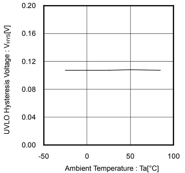
Figure 27. UVLO Hysteresis Voltage vs Ambient Temperature
