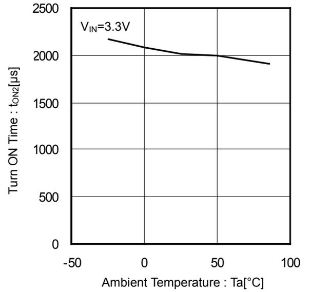
Figure 21. Output Turn ON Time vs Ambient Temperature
