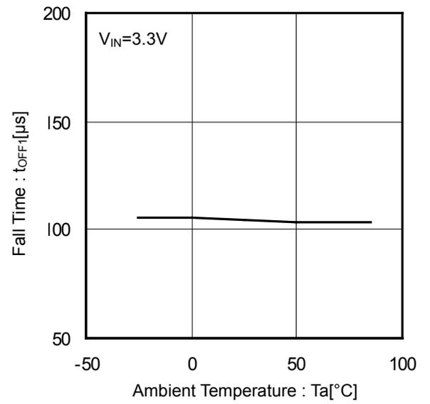
Figure 23. Output Fall Time vs Ambient Temperature
