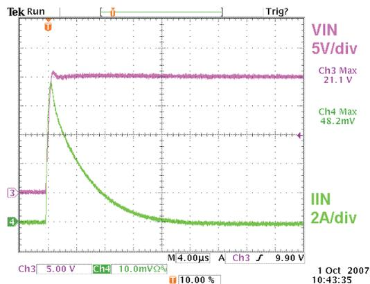
Figure 40. Adapter DC Side Hot Plug-in Test Waveforms
