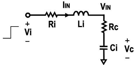
Figure 37. Simplified Equivalent Circuit During Adapter Insertion
