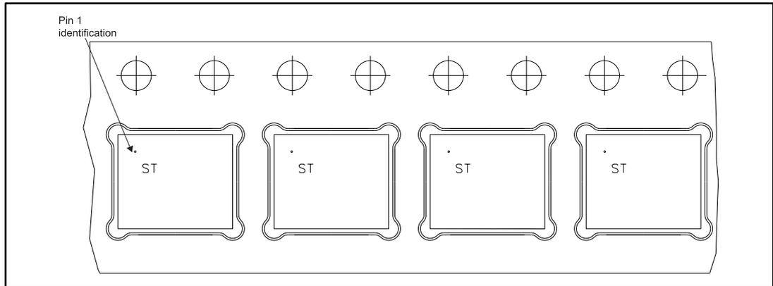
Figure 23: PowerFLAT™ 5x6 reel (dimensions are in mm)
