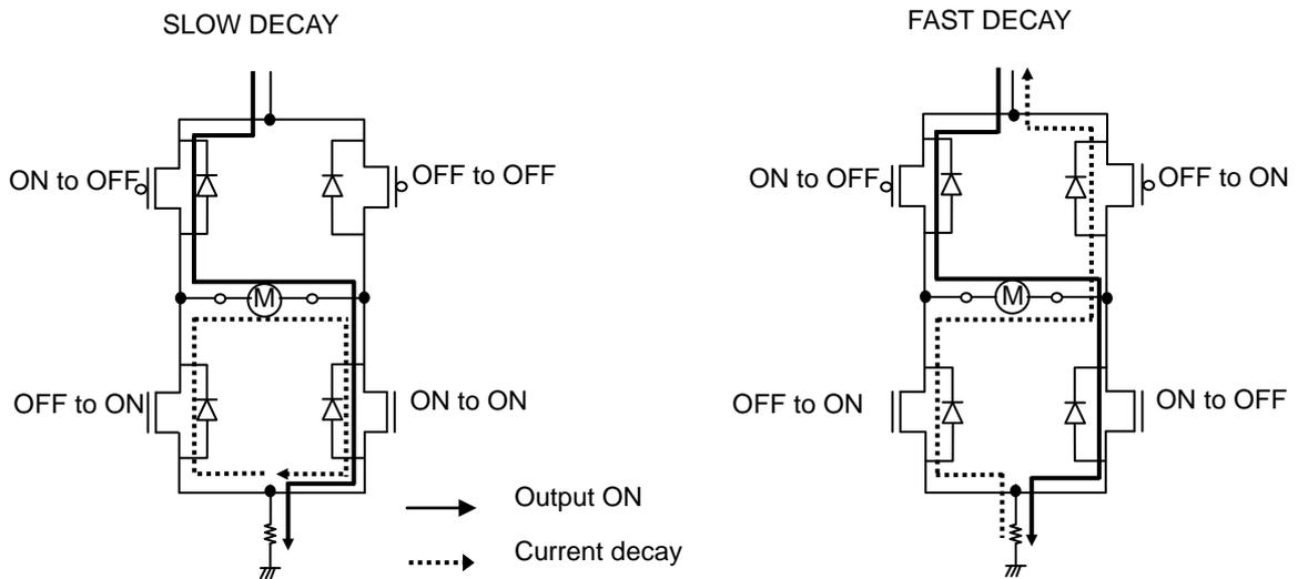
Figure 5. Route of Regenerative Current during Current Decay
