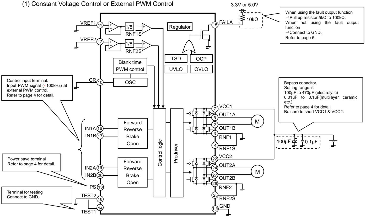
Figure 11. Block Diagram & Application Circuit Diagram
