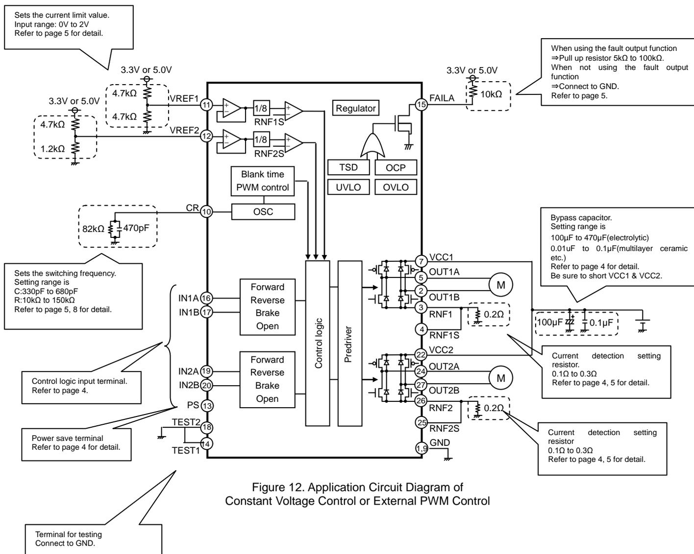
Figure 12. Application Circuit Diagram of Constant Voltage Control or External PWM Control
