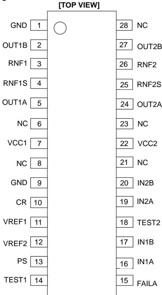
Figure 3. Pin Configuration
