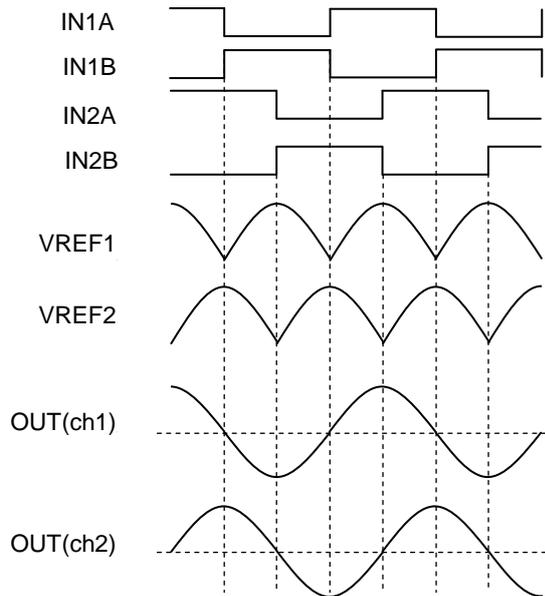
Figure 9.  $\mu$ STEP Control Sequence and Output Current
