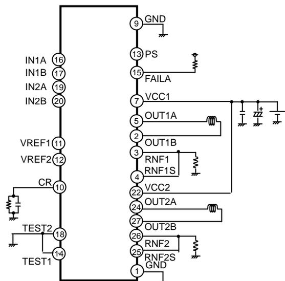
Figure 2. Typical Application Circuit
