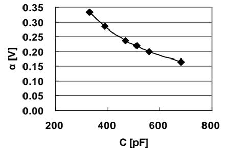
Setting range: C (330pF to 680pF), R (10k $\Omega$  to 150k $\Omega$ )
