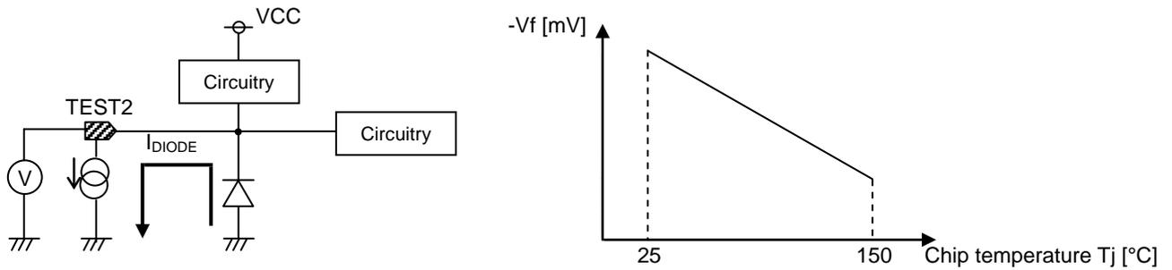
Figure 10. Model Diagram for Measuring Chip Temperature
