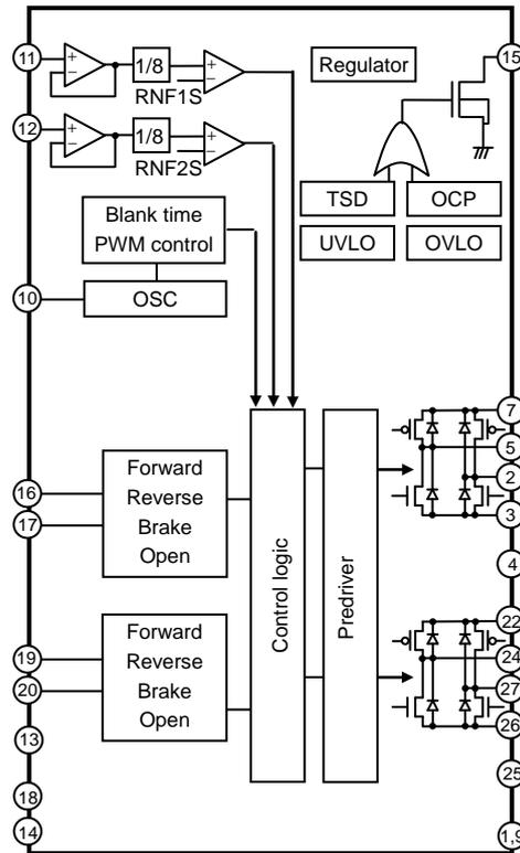
Figure 4. Block Diagram
