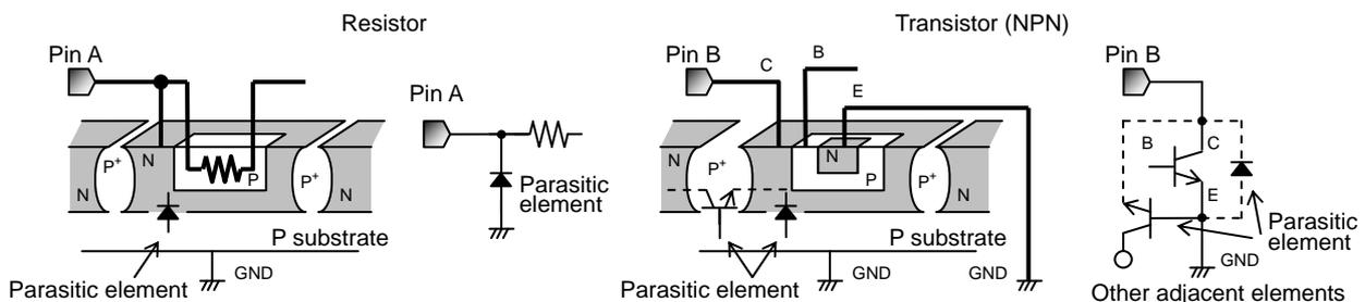
Fig.3 Example of Monolithic IC Structure
