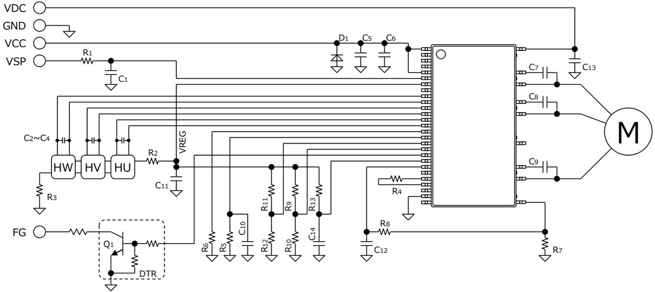
Figure 48. Application Example (180° Sinusoidal Commutation Driver, CCW="H", FGS="H")
