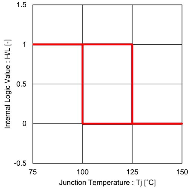
Figure 43 Thermal Shutdown
