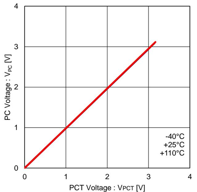
Figure 33. PCT vs PC Linearity
