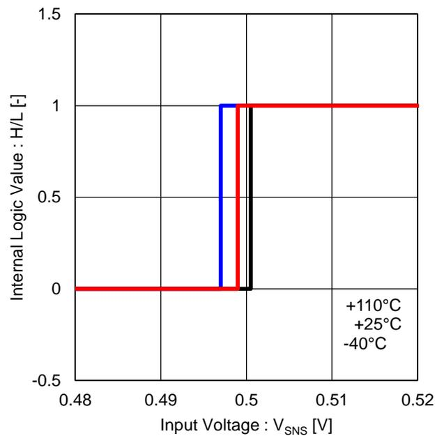
Figure 41. Current Limiter Input Threshold Voltage (SNS)
