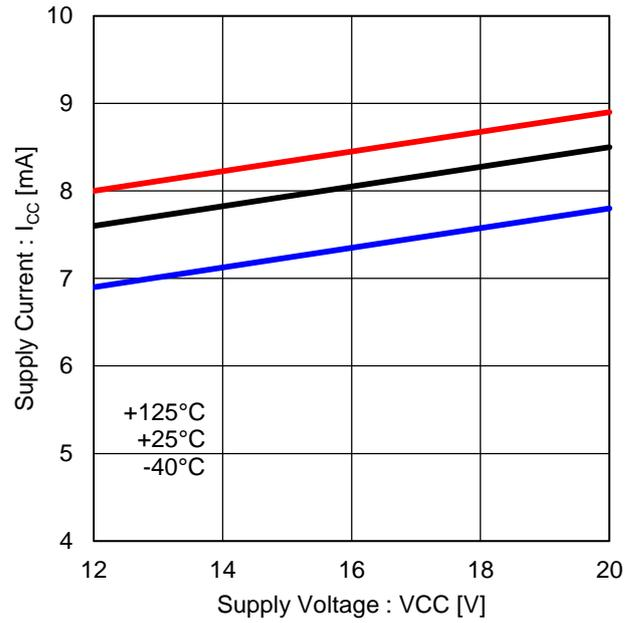
Figure 15. Low Side Drivers Operating Current (F<sub>PWM</sub>: 20kHz)
