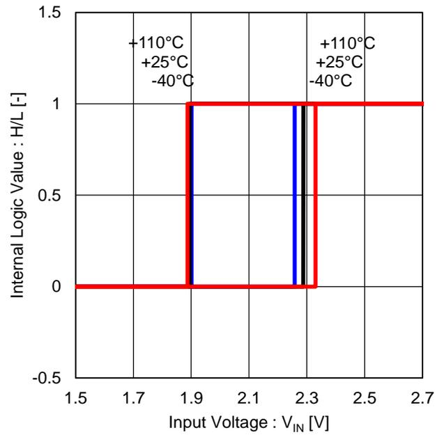
Figure 39. Input Threshold Voltage (CCW, FGS, FOB)
