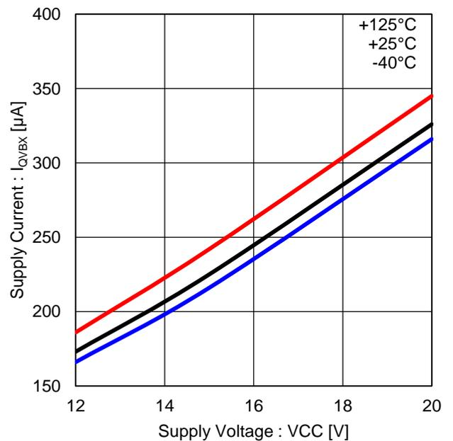
Figure 17. High Side Driver Operating Current (f<sub>PWM</sub>: 20kHz, Each Phase)
