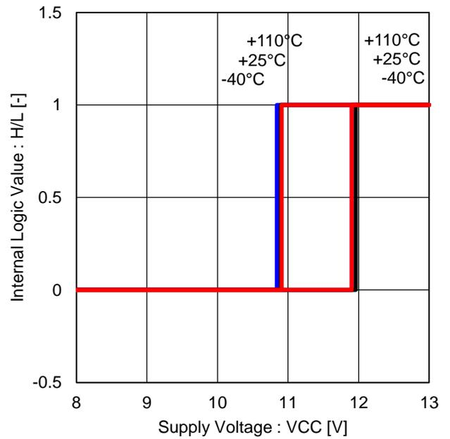
Figure 45. Under Voltage Lock Out (Low Side Drivers)
