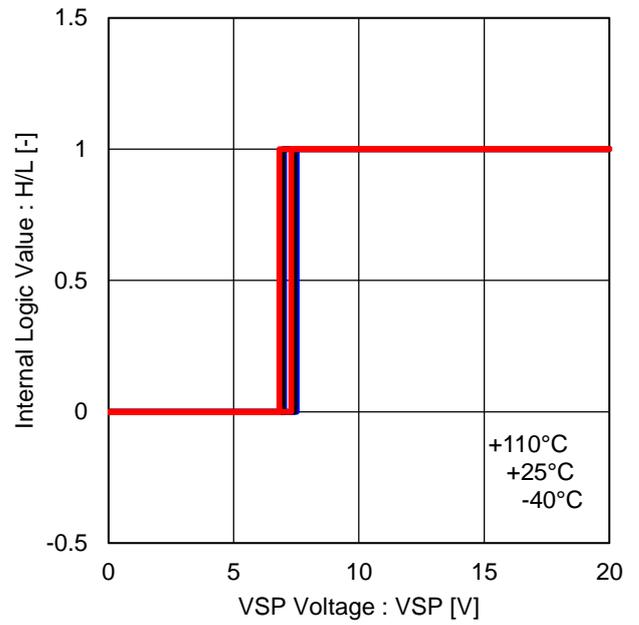
Figure 31. Testing Mode Threshold Voltage
