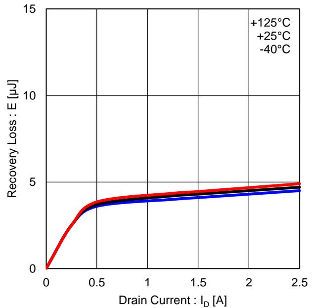
Figure 25. Low Side Recovery Loss (VDC=300V)
