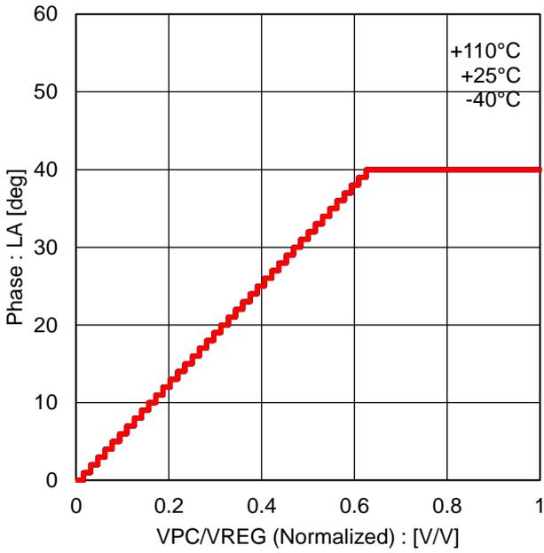
Figure 34. PC Voltage Normalized vs Lead Angle
