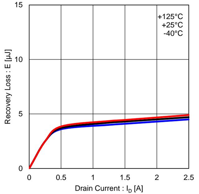
Figure 23. High Side Recovery Loss (VDC=300V)
