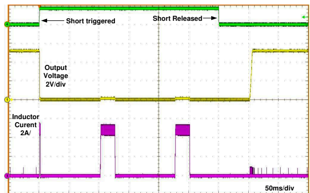
图 7-6. Short-Circuit Transient and Recovery
