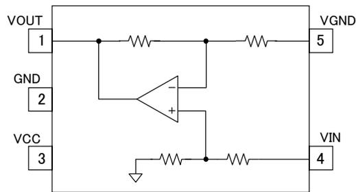
•I/O equivalent circuit diagrams
