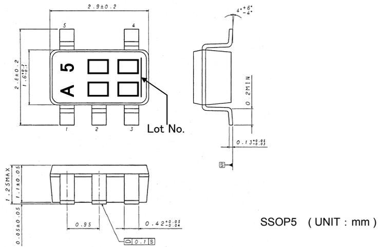
Fig.30 External Dimensions of BH7673G Package
