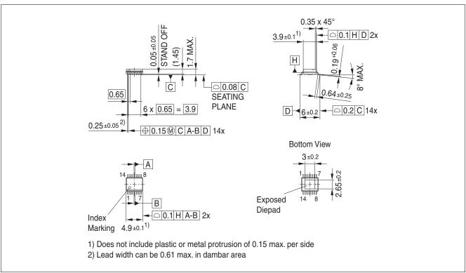
Figure 11 PG-SSOP-14 Exposed Pad<sup>1)</sup>
