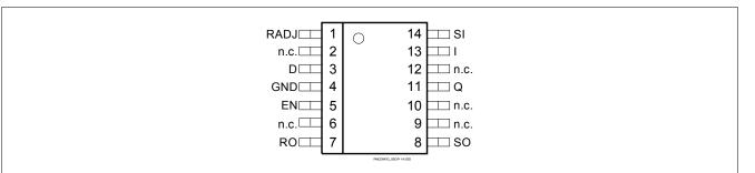
Figure 3 Pin configuration (top view)
