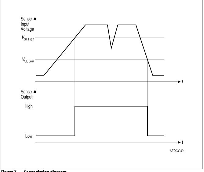
**Figure 7** Sense timing diagram
