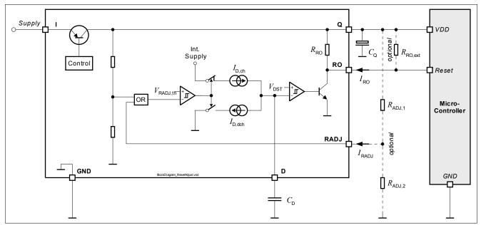
Figure 5 Block diagram reset function
